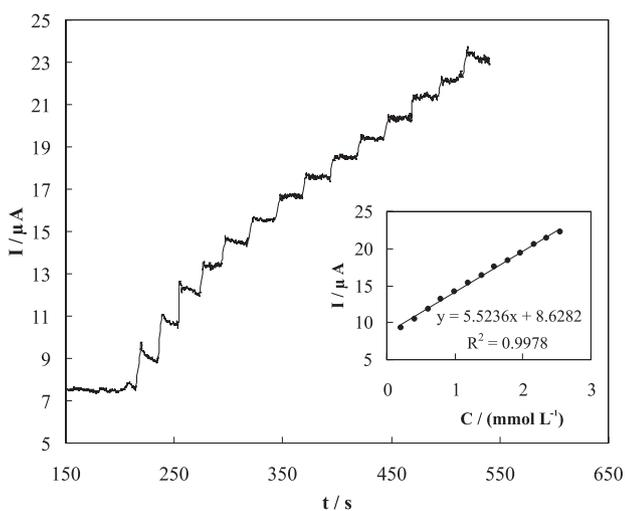
**Figure 4.** Current signal as a function of time in 100 mmol L<sup>-1</sup> sodium hydroxide solution during repetitive injections of etidronate using n-CPE. Applied potential was 610 mV. Inset: Dependency of the transient current on etidronate concentration using n-CPE.
