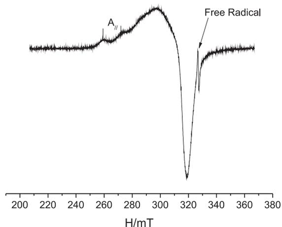
**Figure 3.** EPR spectrum of the SHA sample complexed with copper: T = 90 K and  $A_{\parallel}$  is hyperfine coupling.
