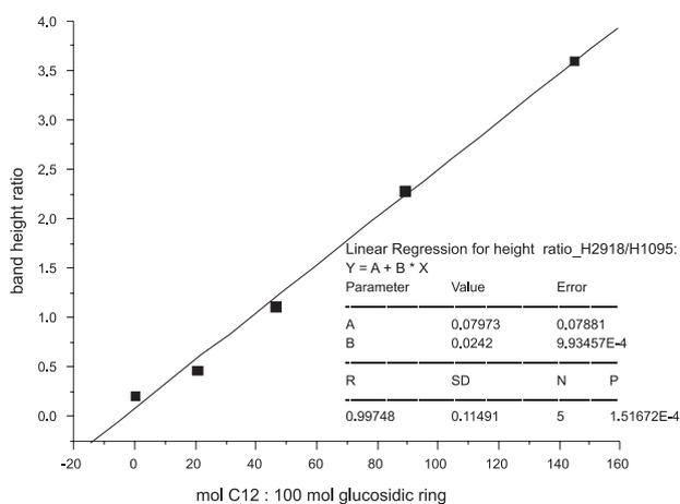
**Figure 4.** Calibration curve based on data Table 2 for the quantitative determination of the degree of insertion. Linear fit of height ratio 2926/1087  $\text{cm}^{-1}$ .
