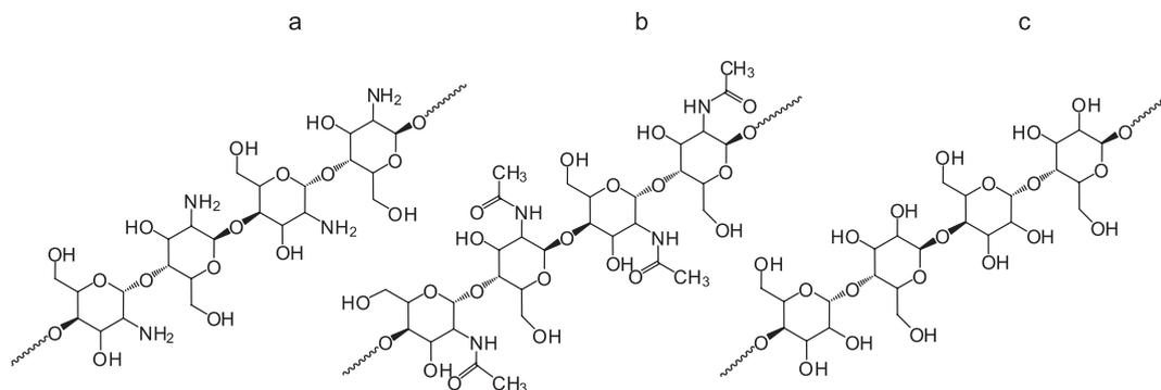
**Figure 1.** Structures of (a) chitosan, (b) chitin, (c) cellulose.
