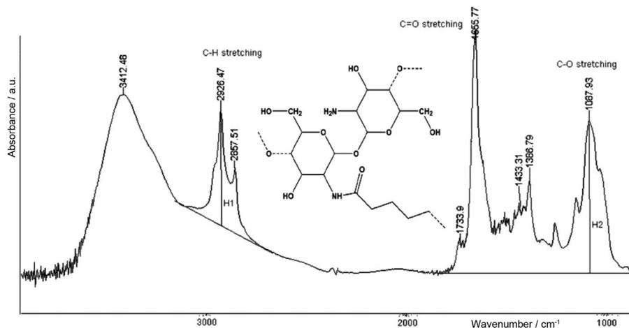
**Figure 3.** FTIR spectrum of grafted chitosan sample with DI = 35%.
