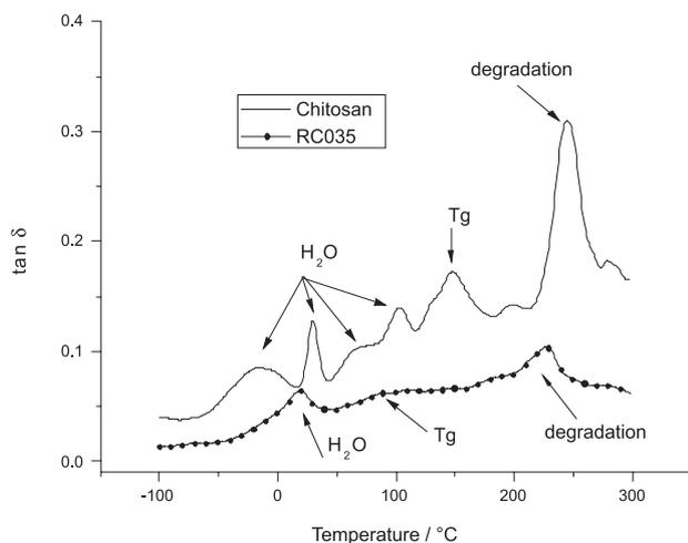
**Figure 8.**  $\tan \delta$  of pristine (solid line) and of substituted chitosan (dotted line) with 44% of degree of insertion.
