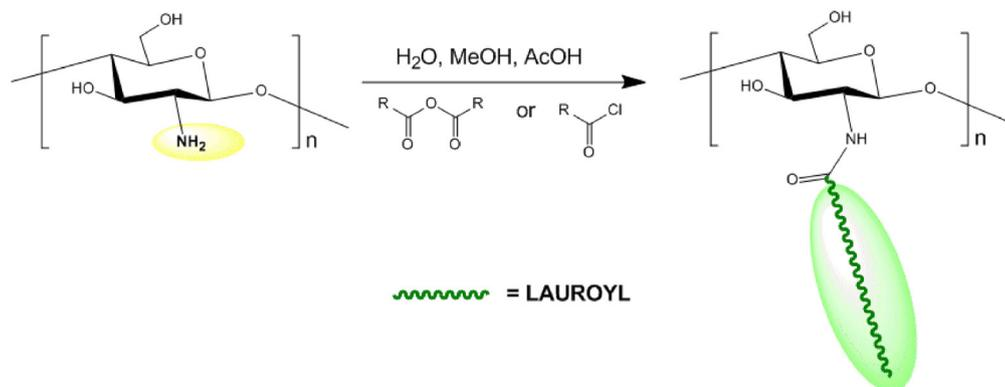
**Figure 2.** Chemical route to the insertion of lauroyl side groups onto the chitosan backbone.
