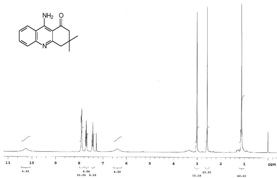
**Figure S9.** <sup>1</sup>H NMR spectrum (300 MHz, CDCl<sub>3</sub>) of compound 17.
