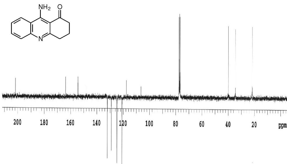
**Figure S8.** <sup>13</sup>C NMR spectrum APT (75 MHz, CDCl<sub>3</sub>) of compound 15.
