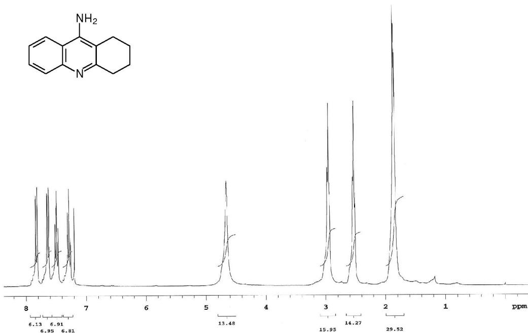
Figure S1. <sup>1</sup>H NMR spectrum (300 MHz, CDCl<sub>3</sub>) of compound 1a.
