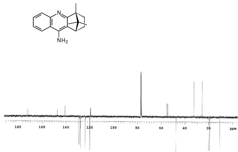
**Figure S12.** <sup>13</sup>C NMR spectrum APT (75 MHz, CDCl<sub>3</sub>) of compound **19**.
