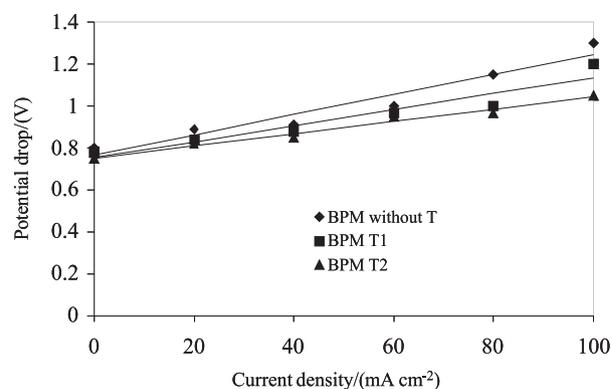
**Figure 6.** Voltage-current characteristics for bipolar membrane in 1 mol L<sup>-1</sup> HCl / 1 mol L<sup>-1</sup> NaOH at room temperature.
