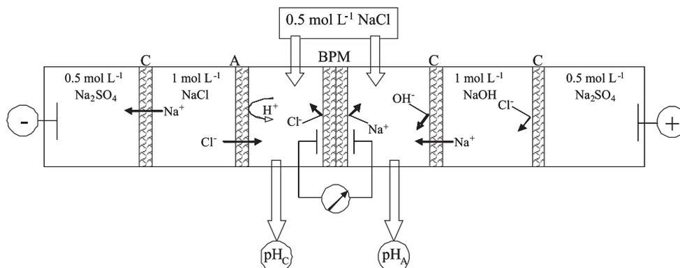
**Figure 5.** Cell with recirculating flows used for membrane stability studies (B = bipolar membrane; C = cation exchange membrane; A = anion exchange membrane).
