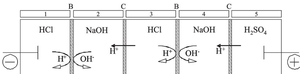
**Figure 4.** Static cell used for membrane characterization studies (B = bipolar membrane; C = cation exchange membrane).
