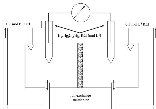
**Figure 3.** Diagram of the test cell used to determine the permselectivity of ion-exchange membranes.
