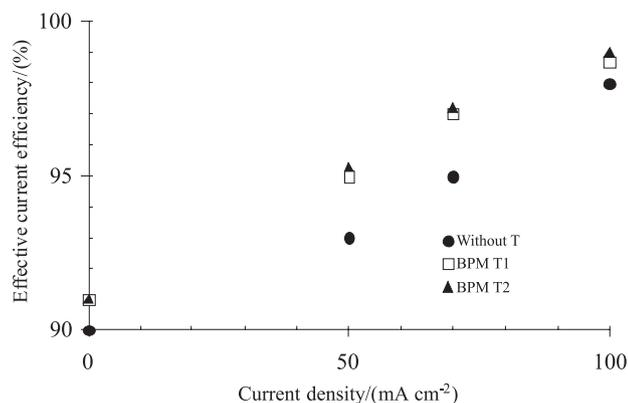
**Figure 8.** Effective current efficiency ( $E'$ ) of a bipolar membrane with and without treatment, at different membrane currents. The membrane separated 1 mol L<sup>-1</sup> HCl / 1 mol L<sup>-1</sup> NaOH solutions at room temperature.
