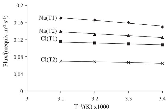
**Figure 10.** Na<sup>+</sup> and Cl<sup>-</sup> ion fluxes versus reciprocal temperature for PVA/PASA-PVA/PDDAB T1 and PVA/PASA-PVA/PDDAB T2 bipolar membranes separating 1 mol L<sup>-1</sup> HCl / 1 mol L<sup>-1</sup> NaOH solutions. The current density was 100 mA cm<sup>-2</sup>.
