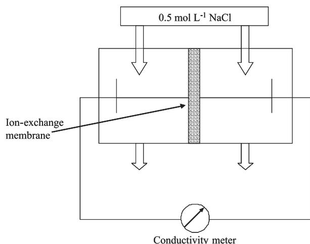
**Figure 2.** Schematic diagram of the test cell used to determine the electrical resistance of ion-exchange membranes.
