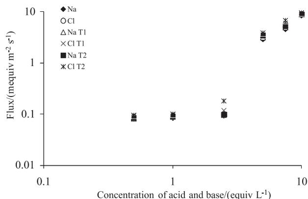
**Figure 9.** Na<sup>+</sup> and Cl<sup>-</sup> ion flux data for different acid/base concentrations at room temperature. The current density was 100 mA cm<sup>-2</sup>.
