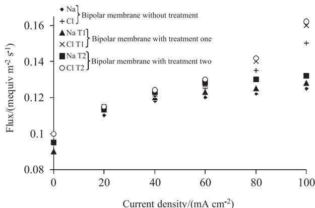
**Figure 7.** Fluxes of Na<sup>+</sup> and Cl<sup>-</sup> ions through bipolar membrane at different current densities. The membrane separated 1 mol L<sup>-1</sup> HCl and 1 mol L<sup>-1</sup> NaOH solutions, at room temperature.
