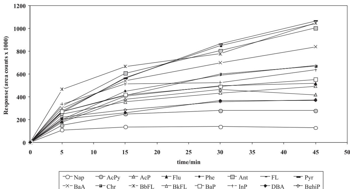
**Figure 3.** Comparison of extraction of PAHs between different extraction times with 30  $\mu\text{m}$  PDMS fibre at an extraction temperature of 60 °C.
