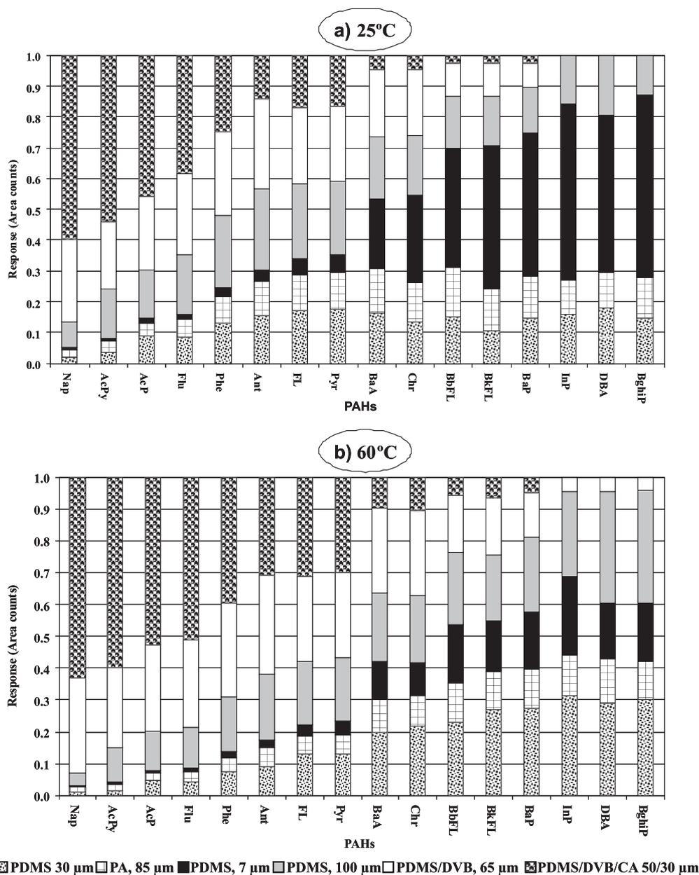
**Figure 2.** Comparison of response of SPME-GC-FID analysis with different fibres coatings at 25 °C (a) and 60 °C (b).
