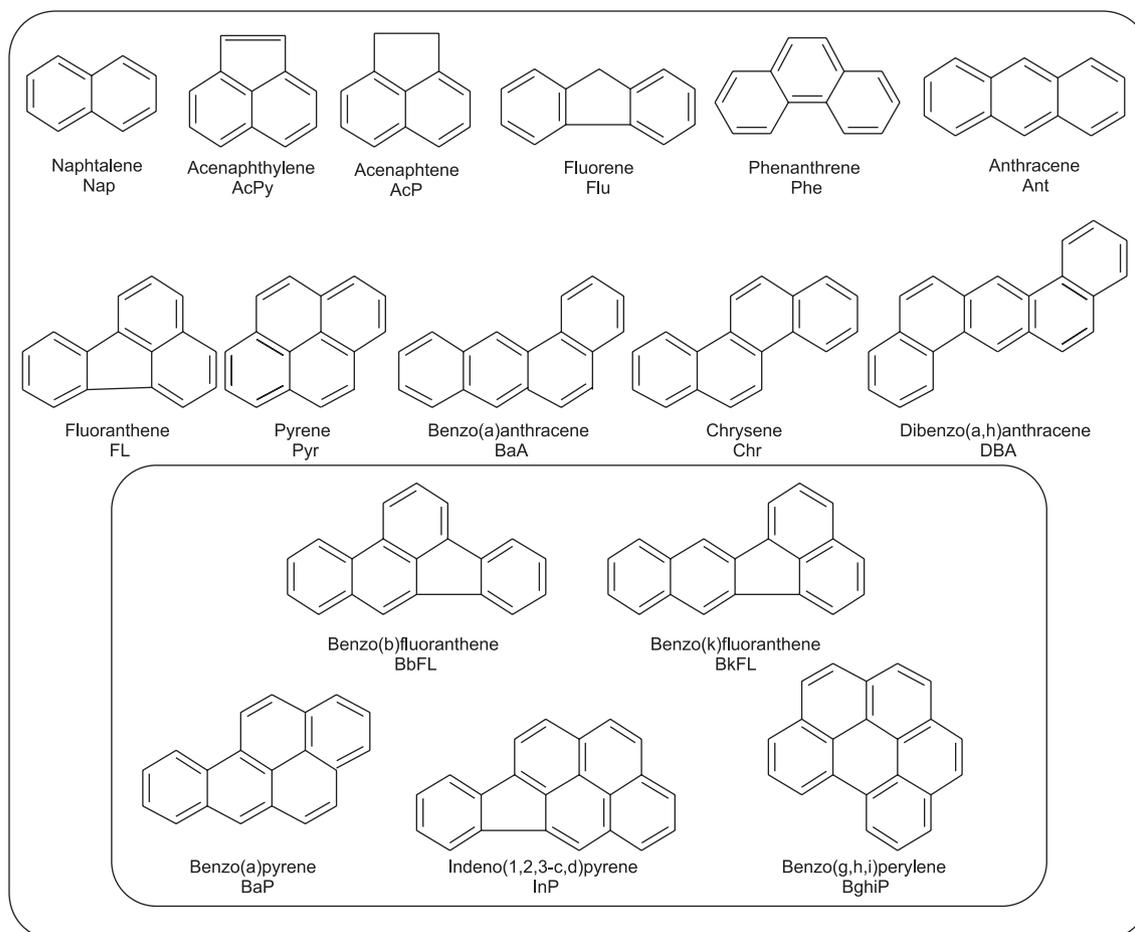
**Figure 1.** Structures of the sixteen PAH studied in this work. The five structures in the small box are the compounds listed in the European Council Directive 98/83/EC. Under each chemical structure are the compound name and its acronym.
