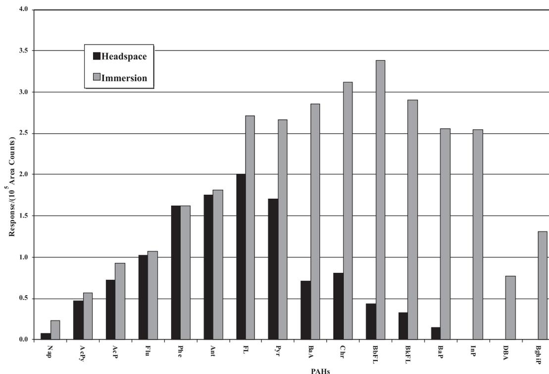
**Figure 6.** Comparison of extraction of PAHs from samples between immersion and headspace SPME at 60 °C during 30 min with a 30  $\mu$ m PDMS fibre and 1500 rpm.
