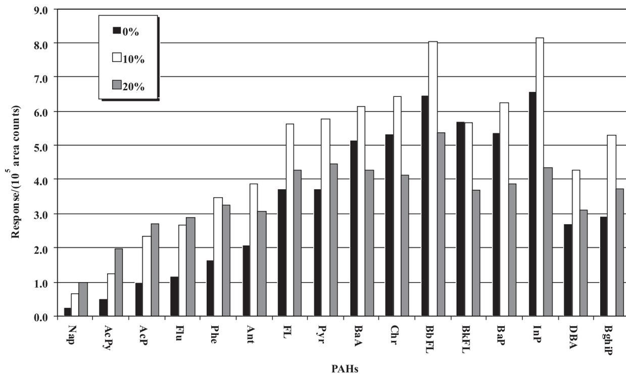
Figure 5. Comparison of extraction of PAHs from samples with different concentrations of NaCl by SPME at 60 °C during 30 min with a 30 μm PDMS fibre.
