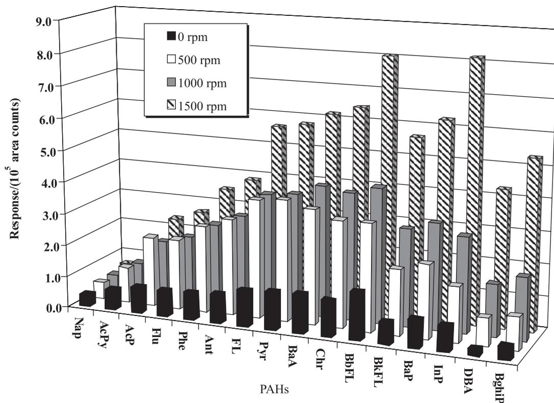
Figure 4. Comparison of extraction of PAHs between static and stirred samples at different speeds by SPME at 60 °C during 30 min with a 30 μm PDMS fibre.
