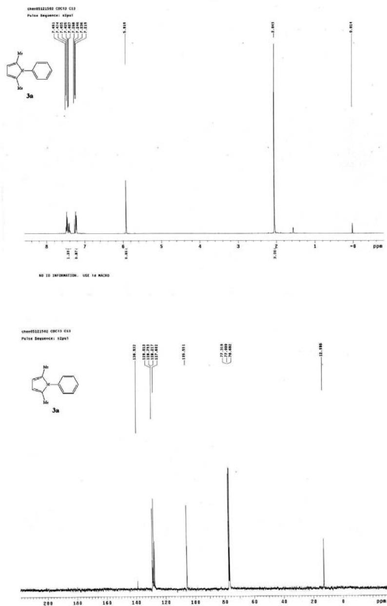
Figure S1.  $^1\text{H}$  NMR of **3a** (400 MHz,  $\text{CDCl}_3$ ) and  $^{13}\text{C}$  NMR of **3a** (100 MHz,  $\text{CDCl}_3$ ).
