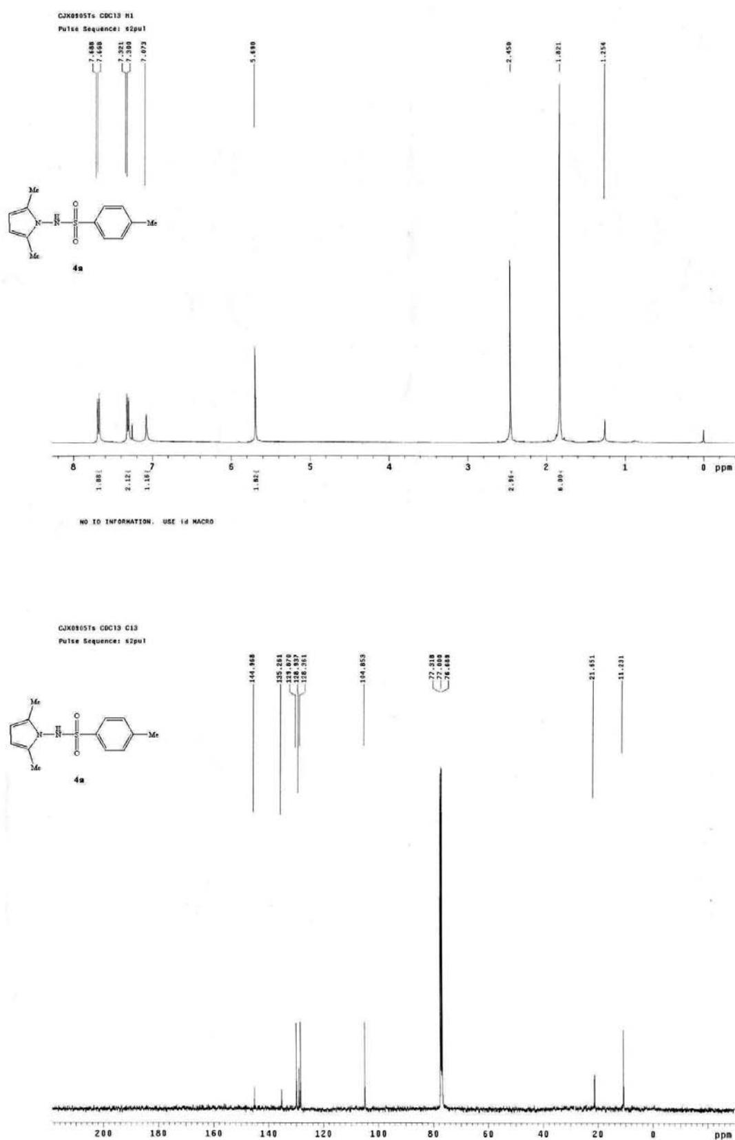
**Figure S24.** <sup>1</sup>H NMR of **4a** (400 MHz, CDCl<sub>3</sub>) and <sup>13</sup>C NMR of **4a** (100 MHz, CDCl<sub>3</sub>).
