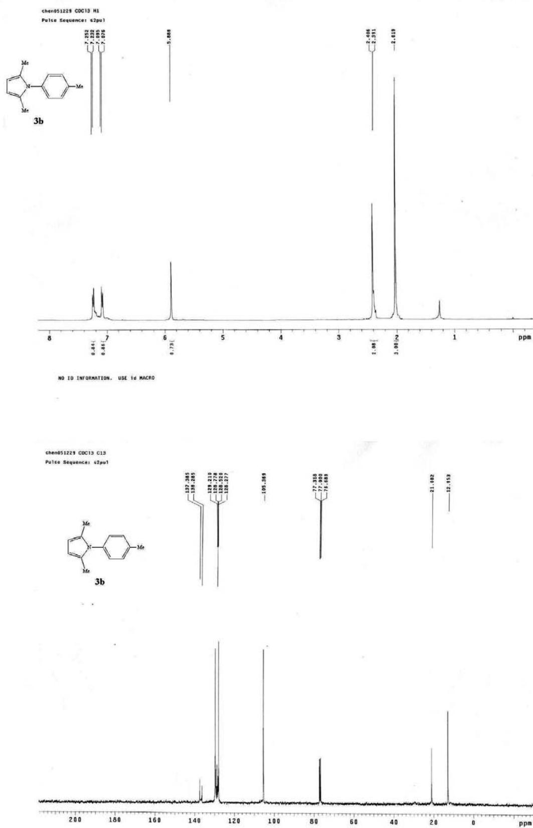
**Figure S2.** <sup>1</sup>H NMR of **3b** (400 MHz, CDCl<sub>3</sub>) and <sup>13</sup>C NMR of **3b** (100 MHz, CDCl<sub>3</sub>).
