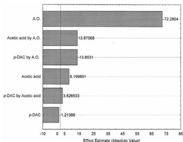
**Figure 2.** Standardized effects of *p*-DAC concentration, acetic acid concentration and addition order of the reagents and their interaction effects on the reflectance measurements ( $\lambda = 510$  nm).
