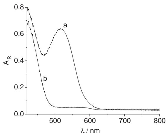
**Figure 1.** Reflectance spectrum a: orange product (conditions: 20  $\mu\text{L}$  *p*-DAC 0.8 % (m/v); 20  $\mu\text{L}$  glacial acetic acid and 10  $\mu\text{L}$  dipyrone  $1.42 \times 10^{-3}$  mol  $\text{L}^{-1}$ ) b: blank (conditions: 20  $\mu\text{L}$  *p*-DAC 0.8 % (m/v); 20  $\mu\text{L}$  glacial acetic acid and 10  $\mu\text{L}$   $\text{H}_2\text{O}$ ). Measurements carried out at 25 °C.
