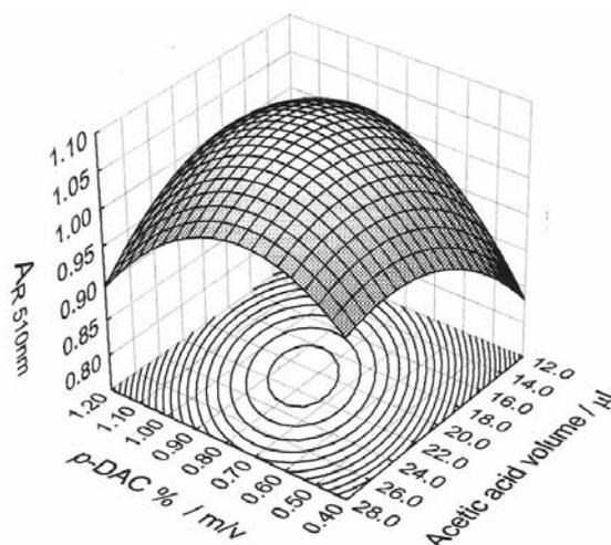
**Figure 3.** Three-dimensional plot of the optimized surface response of reflectance measurements at variable *p*-DAC concentration and glacial acetic acid volume.
