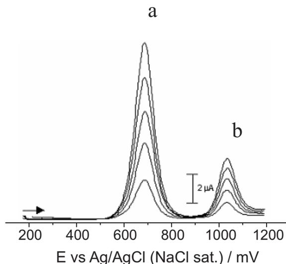
**Figure 4.** Differential pulse voltammograms obtained using the MCPE containing 20% m/m  $\text{PbO}_2$  for L-dopa (a) and carbidopa (b) solutions at concentration ranges from  $2.6 \times 10^{-4}$  to  $1.2 \times 10^{-3} \text{ mol L}^{-1}$  and from  $3.2 \times 10^{-5}$  to  $1.5 \times 10^{-4} \text{ mol L}^{-1}$  in  $0.1 \text{ mol L}^{-1}$  perchloric acid solution, respectively.
