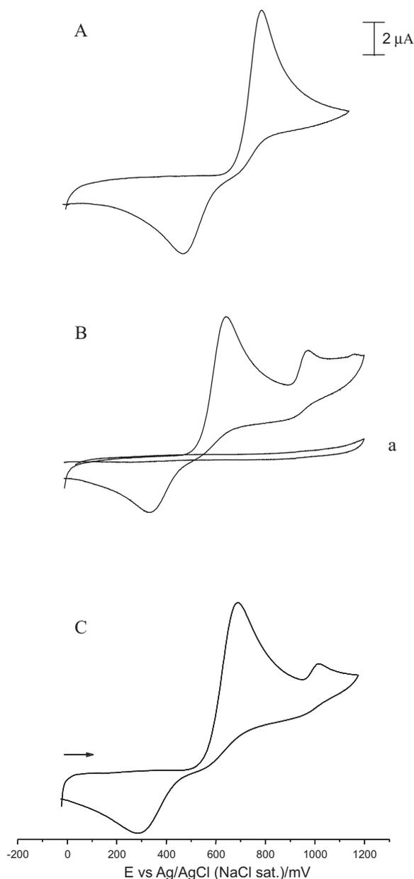
**Figure 1.** Cyclic voltammograms of (A) 5.0 × 10<sup>-4</sup> mol L<sup>-1</sup> L-Dopa, (B) 3.0 × 10<sup>-4</sup> mol L<sup>-1</sup> carbidopa and (C) 1.25 × 10<sup>-3</sup> mol L<sup>-1</sup> L-dopa and 1.25 × 10<sup>-4</sup> mol L<sup>-1</sup> carbidopa in 0.1 mol L<sup>-1</sup> HClO<sub>4</sub> solution obtained using MCPE (b) with 20% m/m PbO<sub>2</sub> at 25 °C and n = 50 mV s<sup>-1</sup>.
