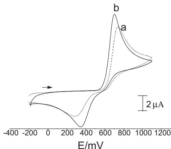
**Figure 2.** Cyclic voltammogram obtained for 5.0 × 10<sup>-4</sup> mol L<sup>-1</sup> L-dopa 0.1 mol L<sup>-1</sup> perchloric acid solution using the CPE (cyclic voltammogram a) and MCPC with 20% m/m PbO<sub>2</sub>. (cyclic voltammogram b) at 25 °C and n = 50 mV s<sup>-1</sup>.
