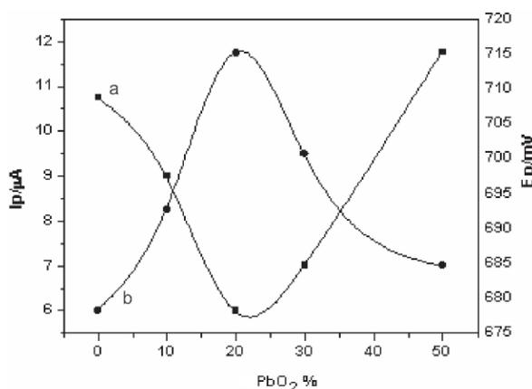
**Figure 3.** Dependence of peak potential (curve a) and peak current (curve b) as a function of the  $\text{PbO}_2$  content in the carbon paste at scan rate of  $5.0 \text{ mV s}^{-1}$ , pulse amplitude of  $50 \text{ mV}$  and scan rate increment of  $3 \text{ mV}$  and  $25^\circ \text{C}$ .
