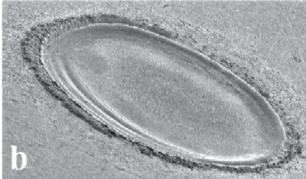
**Figure 5.** Photographs of aluminum samples showing the ablation craters produced by (a) one pulse and (b) one thousand consecutive laser pulses.
