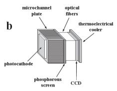
Figure 7. Illustrations of (a) an echelle spectrograph and its generated bidimensional dispersion and (b) a bi-dimensional ICCD.
