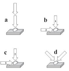
**Figure 6.** Schematic representations of different double-pulse configurations: (a) collinear, (b) orthogonal re-heating, (c) orthogonal pre-ablation and (d) crossed beam (the arrows represent the direction of propagation and the numbers represent the temporal sequence of the two laser pulses).
