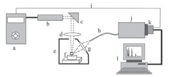
**Figure 1.** Schematic diagram of a simple LIBS system.(a) laser source and cooler; (b) pulsed laser head; (c) mirror; (d) focusing lens; (e) excitation chamber; (f) sample; (g) collecting optics; (h) optical fiber; (i) detector trigger signal; (j) wavelength selector; (k) detector array and (l) microcomputer.
