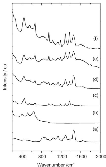
**Figure 1.** Raman spectra. (a) U(600); (b) Hydrolyzed Ti(OPr<sup>i</sup>)<sub>4</sub> heat-treated at 300 °C for 24 h; (c) acac stabilized Ti<sup>4+</sup> sol dried at 80 °C for 2h; (d) U(600)Ti<sub>1</sub>; (e) U(600)Ti<sub>3</sub> and (f) U(600)Ti<sub>5</sub>.
