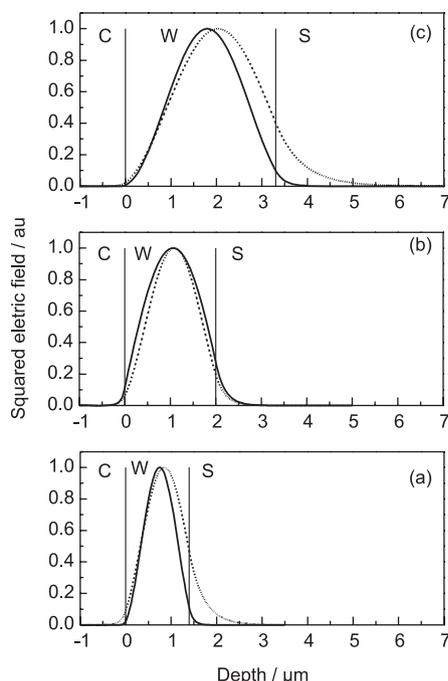
**Figure 7.** Calculated square electric field profiles of the  $TE_0$  mode at 1550 nm (dash line) and 632.8 nm (straight line) of the waveguides across the layered structure-cladding of air C, waveguide W, and the soda-lime substrate S of the planar waveguide.
