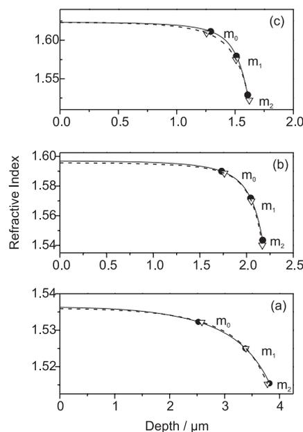
**Figure 6.** Refractive index profiles of the U(600)Ti<sub>1</sub> (a), U(600)Ti<sub>3</sub> (b), and U(600)Ti<sub>5</sub> (c) planar waveguides reconstructed from modal measurements at 632.8 nm for TE (straight line) and TM (dash line) polarization. The effective indices of the TE (•) and TM (∇) modes are reported.
