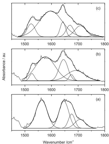
**Figure 3.** FT-IR absorption spectra (deconvolution results). (a) U(600); (b) U(600) $\text{Ti}_1$  and (c) U(600) $\text{Ti}_5$ .
