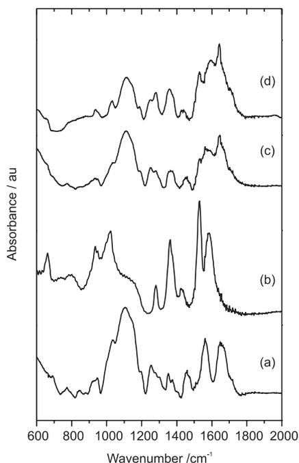
**Figure 2.** FT-IR absorption spectra. (a) U(600); (b) acac stabilized  $\text{Ti}^{4+}$  sol dried at 80 °C for 2h; (c) U(600) $\text{Ti}_1$  and (d) U(600) $\text{Ti}_5$ .
