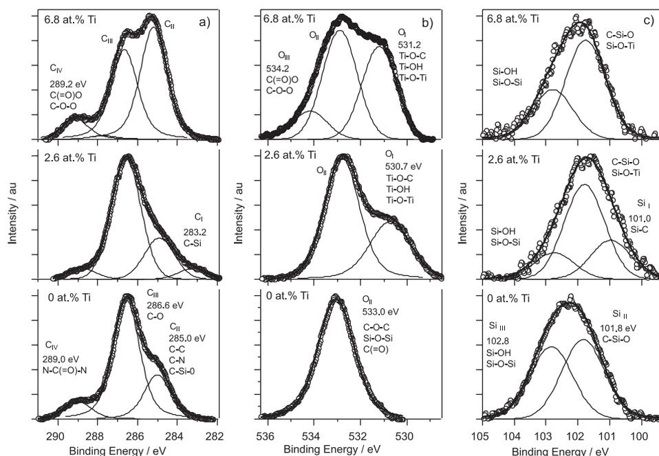
**Figure 4.** XPS deconvoluted C 1s (a), O 1s (b) and Si 2p (c) core-level spectra for the undoped hybrid and titanium-doped samples U(600)Ti<sub>1</sub>, U(600)Ti<sub>3</sub> and U(600)Ti<sub>5</sub>.
