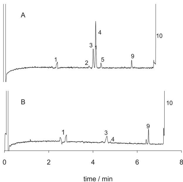
**Figure 3.** Analysis of industrial batches of crude (A) and highly-purified (B) terephthalic acid in regular 75  $\mu\text{m}$  fused-silica capillaries. CTA sample: 5000 mg/L and PTA sample: 10000 mg/L, both in 0.15 mol L<sup>-1</sup> NaOH. Other conditions and peak identification as in Figure 2B.
