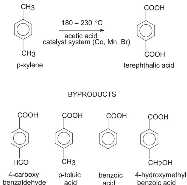
**Figure 1.** Schematic representation of the synthesis of terephthalic acid and chemical structures of the major byproducts.
