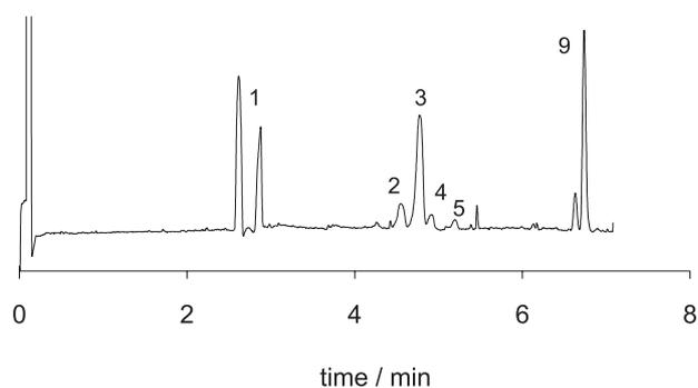
**Figure 4.** Analysis of an industrial batch of highly-purified terephthalic acid in high-sensitivity optical cell. PTA sample: 10000 mg/L in 0.15 mol L<sup>-1</sup> NaOH. Other conditions and peak identification as in Figure 2B.
