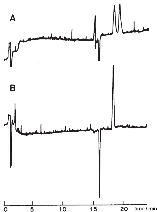
Figure 5. Enantiomeric separation of omeprazole by capillary electrophoresis. (a) commercial tablet of rac-omeprazole; (b) commercial tablet of (S)-omeprazole. Conditions: 3% sulfated \beta -cyclodextrin in 20 mmol L -1 phosphate buffer, pH 4; applied voltage: 20 kV; temperature: 20 °C; hydrodynamic injection (50 mbar, 10 seconds); UV detection at 202 nm.
