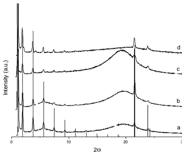
**Figure 3.** Overlay of the column graph representation of XRD data for crystalline **C36** in its  $B_O$  phase<sup>45</sup> and the XRD patterns for gels composed of **C36** at (a) 4 wt% in 1-octanol, (b) 2 wt% in 1-octanol, (c) 4 wt% in hexadecane and (d) 4 wt% in glycidyl methacrylate (adapted from ref 43).
