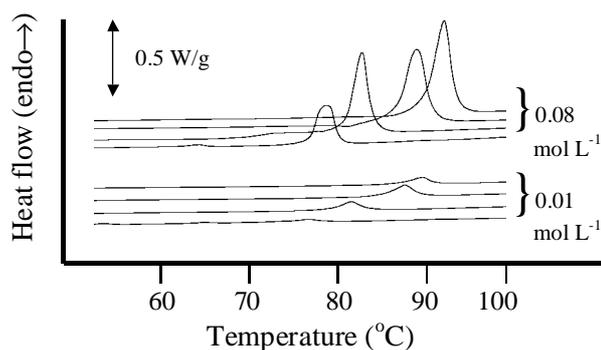
**Figure 1.** DSC heating thermograms of fast-cooled (See Table 1)  $\text{nNBr}$ /hexadecane gels at 0.01 and 0.08  $\text{mol L}^{-1}$  gelator concentrations. The values of  $n$  for each concentration are in the order 12 $\rightarrow$ 14 $\rightarrow$ 16 $\rightarrow$ 18 from bottom to top<sup>37</sup>.
