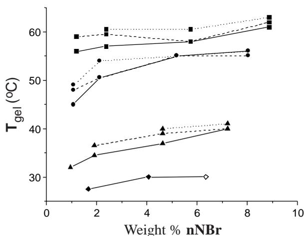
**Figure 2.** The influence of cooling rates of **nNBr**/styrene sols on the  $T_{\text{gel}}$  values of their gels:  $n = 18$  (■),  $16$  (●),  $14$  (▲),  $12$  (◆, ); fast (—), moderate (-----) and slow (.....) cooling; see Table 1. Averages are reported when ranges of melting were noted. The value is the same for fast, moderate and slow cooling<sup>37</sup>.
