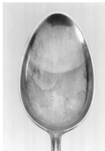
**Figure 5.** Silver spoon coated with TSHP. Just one half of the spoon was coated, while the other half remained uncoated. After this the spoon was immersed in  $H_2S$  saturated medium during 12 hours. Photo taken 8 months after the experiment.
