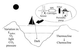
Figure 6. Scheme of a flow manifold for the *in-situ* study of lake chemistry at different deep levels.
