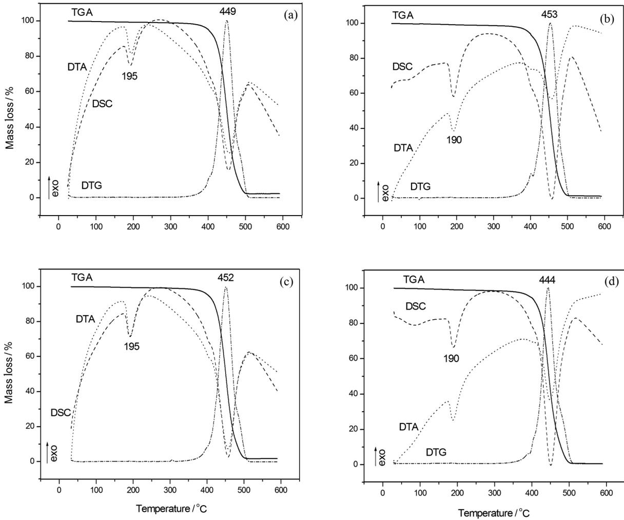
**Figure 4.** Thermal analysis of the NcP after 15 (a) and 30 (b) days in SBF and NsP after 15 (c) and 30 (d) days in SBF.
