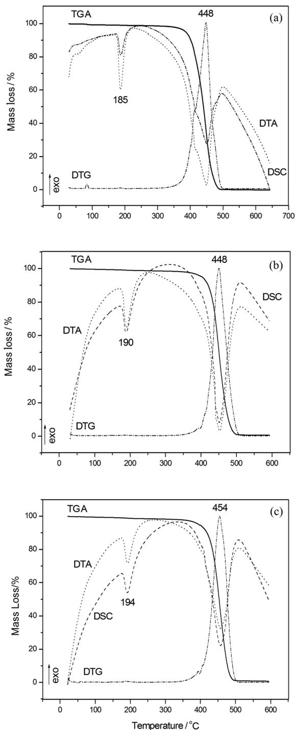
**Figure 3.** Thermal analyses of PA (a), NcP (b) and NsP (c).
