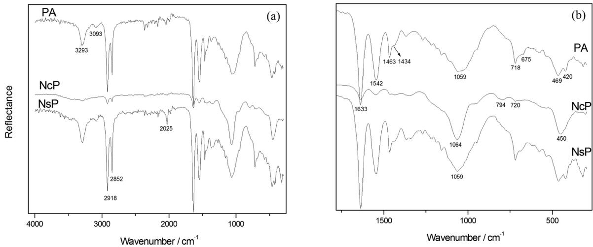
**Figure 5.** ATR-FTIR spectra of the PA, NcP and NsP.
