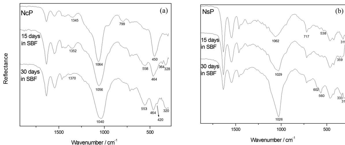
**Figure 6.** ATR-FTIR spectra of the NcP (a) and NsP (b) before and after contact with SBF.**Table 2.** Characteristic wavenumbers for the samples NcP(15), NcP(30), NsP(15) and NsP(30) after contact with the SBF solution for 15 and 30 days
