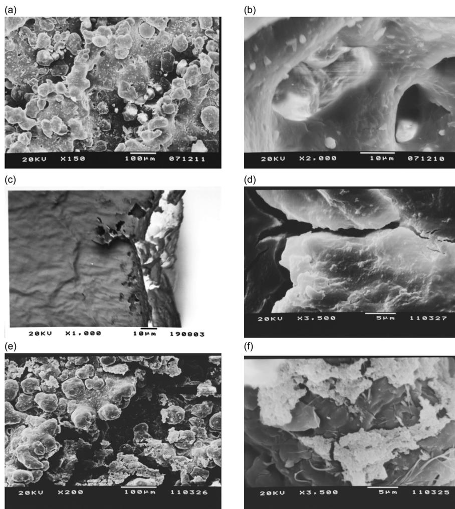
**Figure 1.** Surface of the PA substrate before coating (a and b) and after coating, thickness of the film in NcP (c), NcP surface (d) and NsP surface (e and f).
