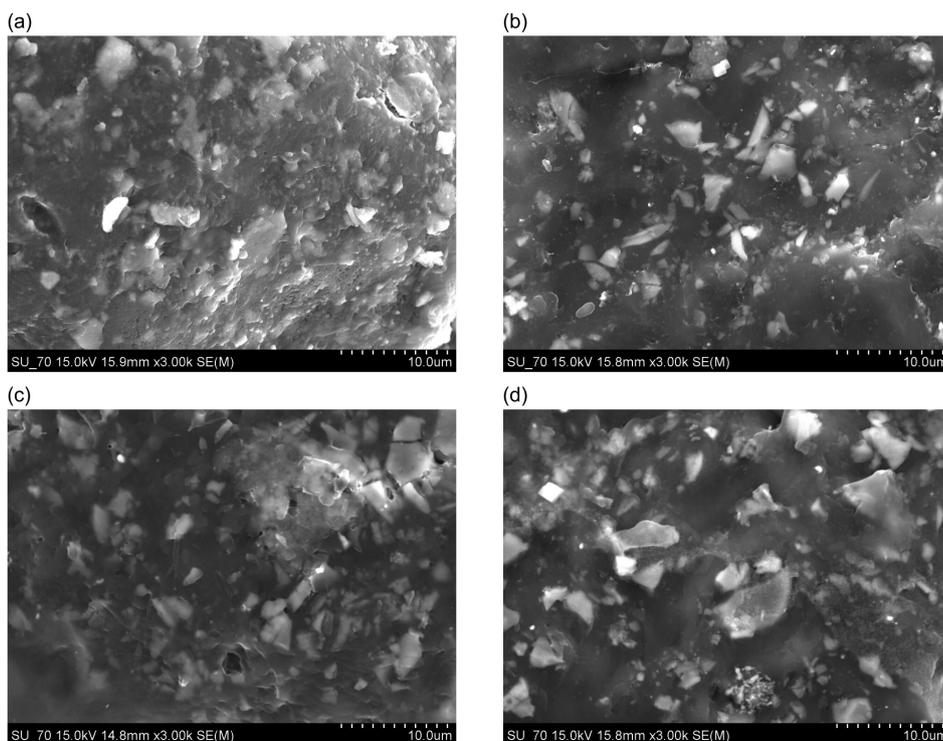
**Figure 2.** Surface of the PA substrate after contact with SBF (a) NcP 15 days, (b) NcP 30 days, (c) NsP 15 days and (d) NsP 30 days.
