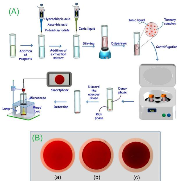
**Figure 1.** (A) Schematic representation of the system for the determination of antimony; (B) images of the rich-phase corresponding to solutions containing  $\text{Sb}^{\text{III}}$  at (a) 0.0; (b) 5.0; and (c) 50.0  $\mu\text{g L}^{-1}$ .
