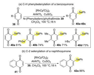
Scheme 10. Phenylselenylation of benzoquinones and 1,4-naphthoquinone (adapted from reference 45).
