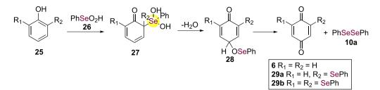
Scheme 6. o-Oxidation of phenols using benzeneselenenyl acid (adapted from reference 41).
