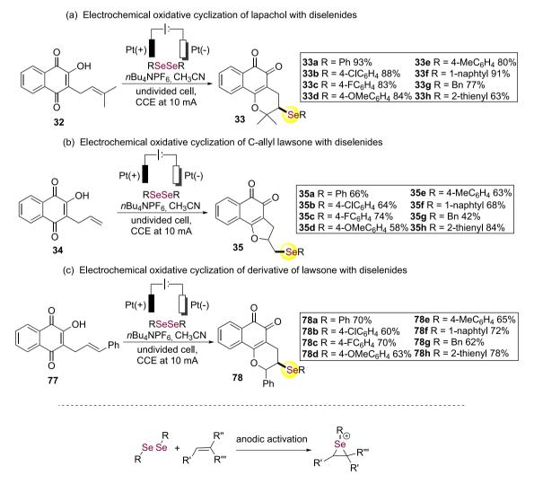
Scheme 20. Electrochemical selenylation/cyclization employing a quinone component (adapted from reference 56).
