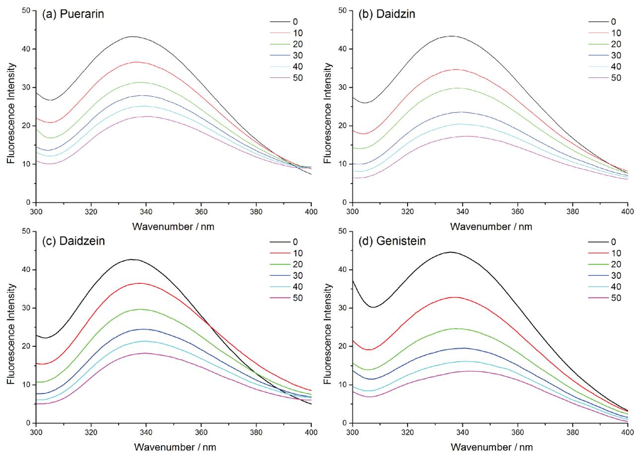
**Figure 4.** The quenching effects of (a) puerarin; (b) daidzin; (c) daidzein and (d) genistein on XO fluorescence spectra.  $\lambda_{\text{exc}} = 280 \text{ nm}$ ;  $1.0 \mu\text{mol L}^{-1}$  XO; the addition of inhibitors was 10, 20, 30, 40 and 50  $\mu\text{mol L}^{-1}$ .
