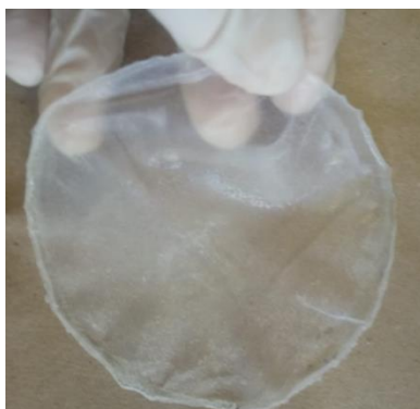
Figure S1. Image of the regenerated cellulose membrane obtained by spreading 7 mL of cellulose solution in 10 cm diameter Petri dish.
