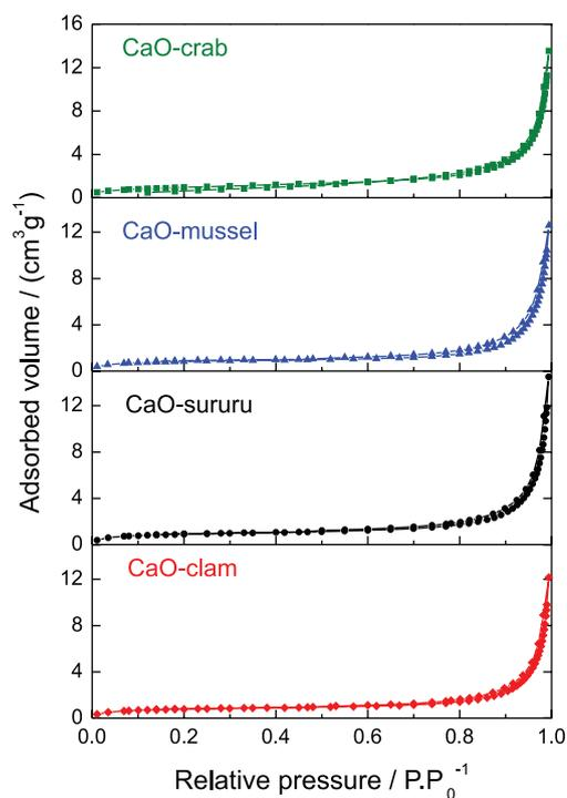
**Figure 4.** Isotherms of nitrogen adsorption and desorption of the CaO catalysts.
