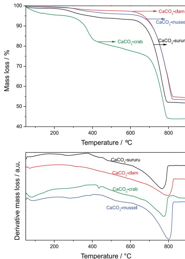
**Figure 1.** TG and derivative thermogravimetry (DTG) curves of fishery residues.
