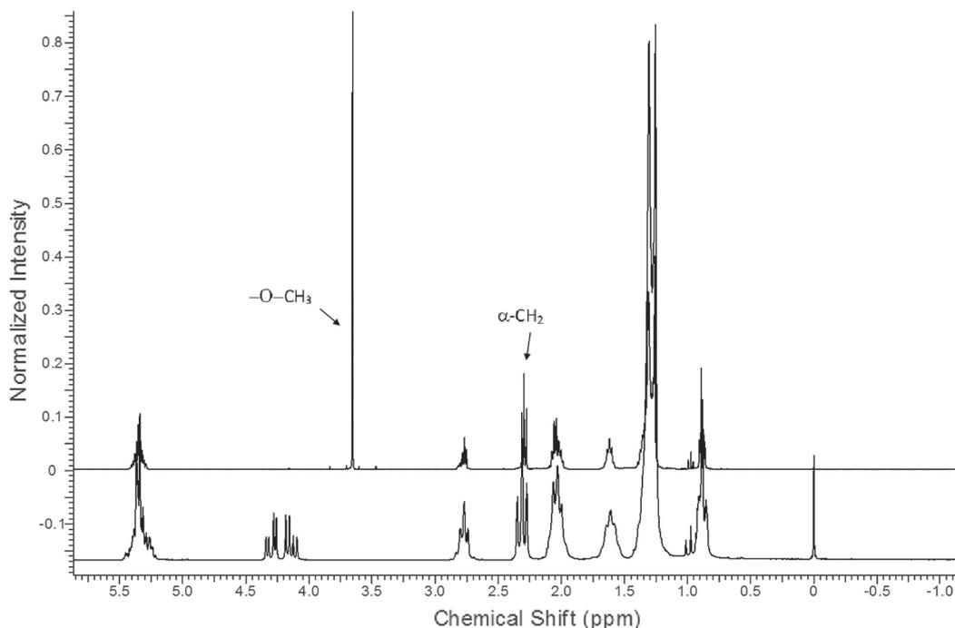
Figure 7.  $^1\text{H}$  NMR (300 MHz,  $\text{CDCl}_3$ ) spectrum of soybean oil and its respective FAME.
