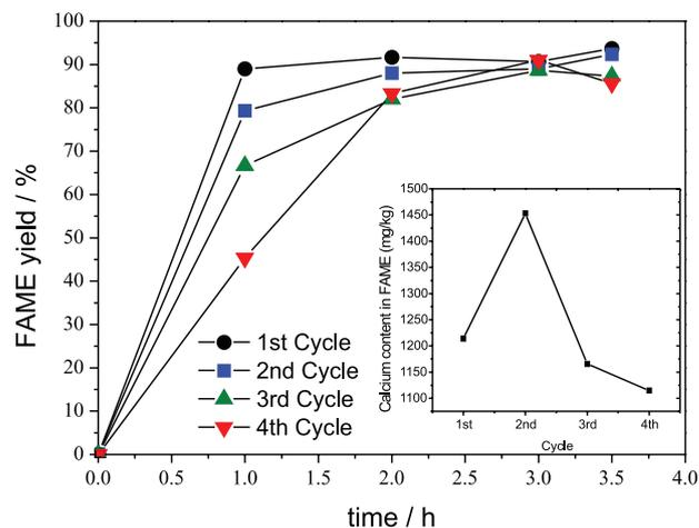
**Figure 9.** FAME yield kinetics for the transesterification of soybean oil over CaO-sururu catalyst during four cycles of reaction and calcium contents in FAME. Insert: the amount of  $\text{Ca}^{2+}$  leached from the CaO-sururu catalyst during the 4 cycles.
