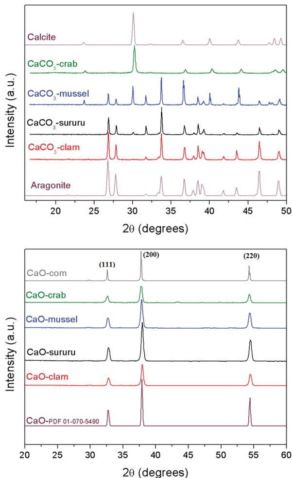
**Figure 2.** Diffractograms of fishery residues before calcination and CaO catalysts.
