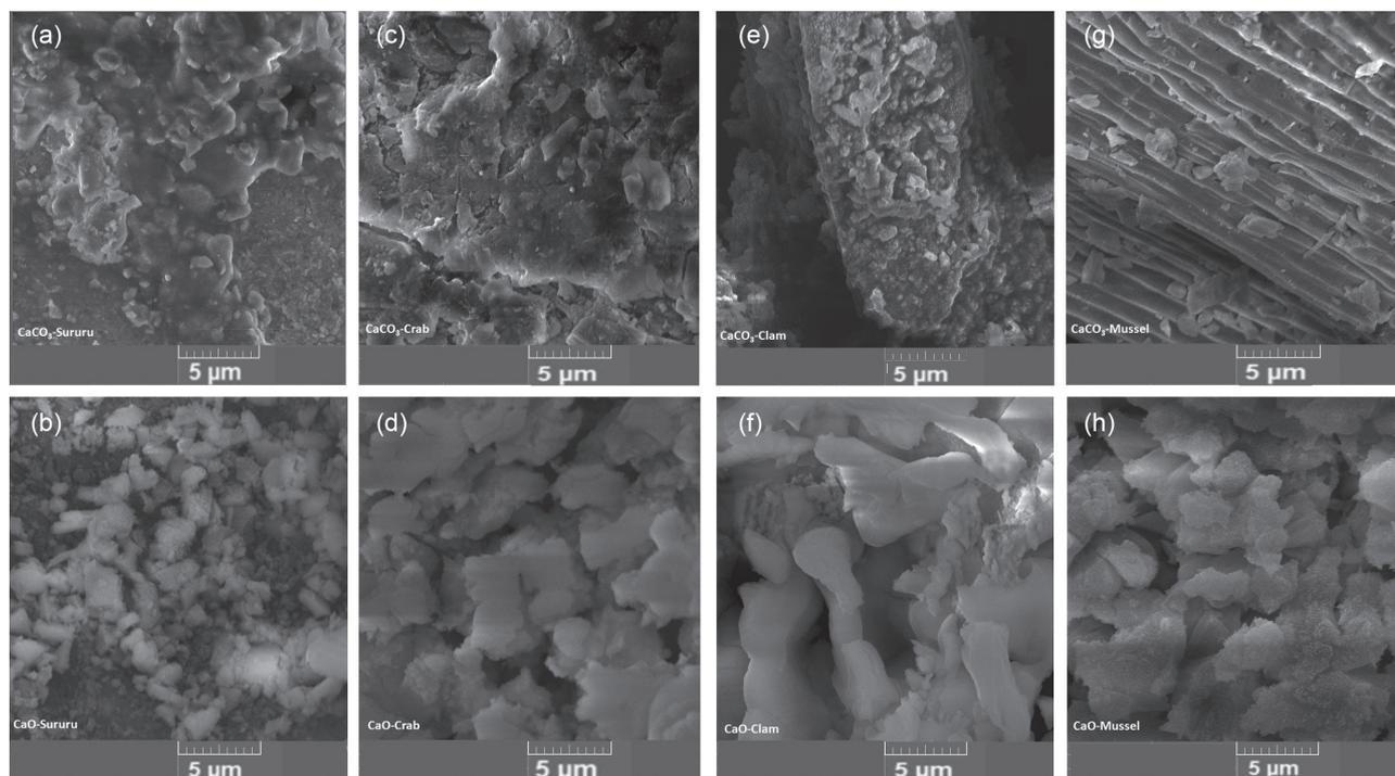
**Figure 5.** SEM micrographs of (a) sururu, (c) crab, (e) clam and (g) mussel fishery residues and CaO (b) sururu, (d) crab, (f) clam and (h) mussel catalysts obtained after calcination.
