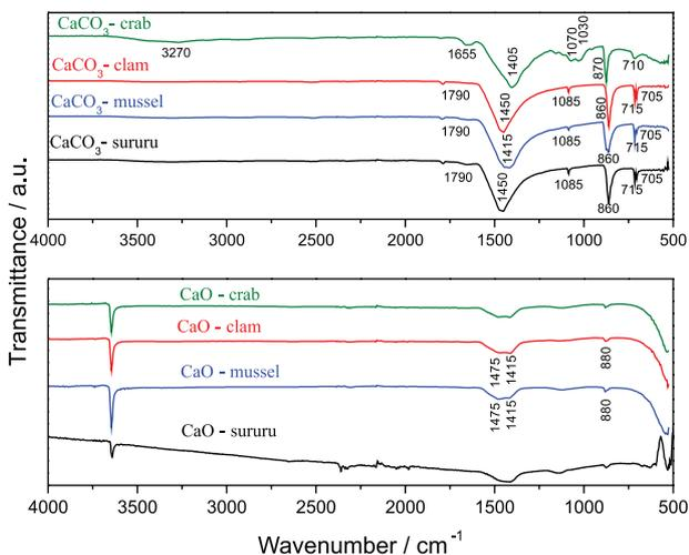
**Figure 3.** FTIR-ATR spectra of uncalcined fishery residues and CaO catalysts.
