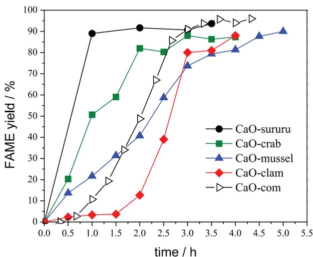
Figure 8. Fatty acid methyl ester (FAME) yields for the transesterification of soybean oil over catalysts. Methanol:oil molar ratio = 18:1, temperature =  $65\text{ }^\circ\text{C}$  at reflux, catalyst concentration = 5 mass%.
