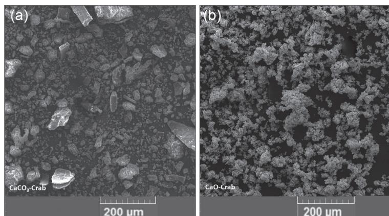
**Figure 6.** SEM comparison of (a)  $\text{CaCO}_3$ -crab shell and (b) CaO-crab catalyst.
