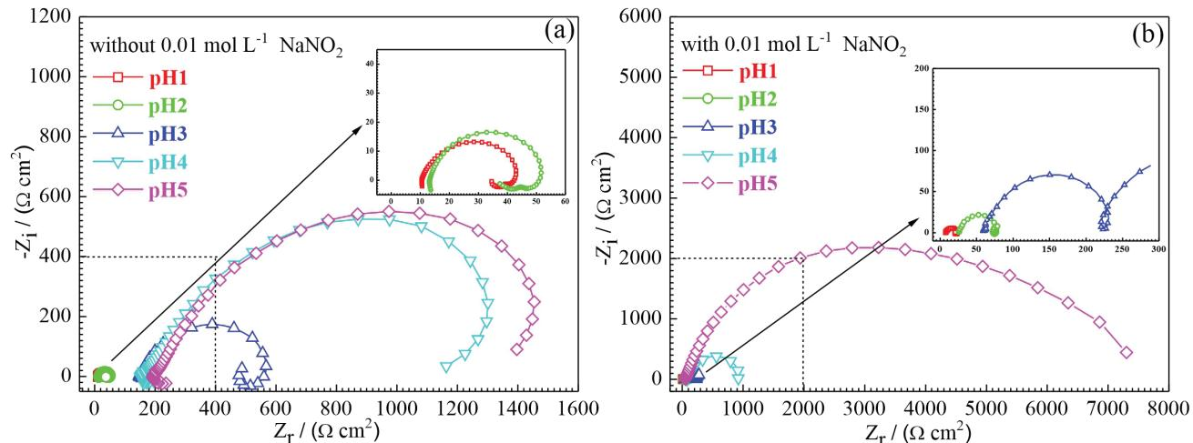
**Figure 5.** EIS of X65 samples in pH 1 to 5  $\text{HNO}_3$  solutions: (a) without  $0.01 \text{ mol L}^{-1}$   $\text{NaNO}_2$  and (b) with  $0.01 \text{ mol L}^{-1}$   $\text{NaNO}_2$ .
