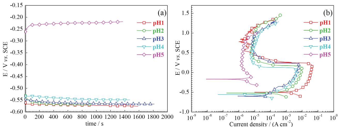
**Figure 4.** OCP evolutions and potentiodynamic polarization curves of X65 samples in pH 1 to 5 HNO<sub>3</sub> solutions with 0.01 mol L<sup>-1</sup> NaNO<sub>2</sub>: (a) OCP and (b) polarization.
