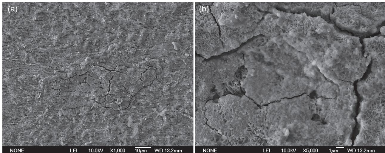
**Figure 3.** Surface SEM morphologies of X65 samples polarized to  $0.5 \text{ V}_{\text{SCE}}$  in pH 3  $\text{HNO}_3$  solutions without  $0.01 \text{ mol L}^{-1} \text{ NaNO}_2$ .
