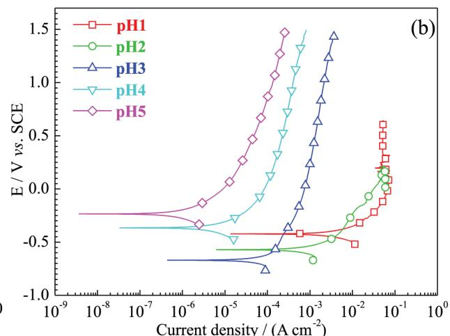
**Figure 2.** OCP evolutions and potentiodynamic polarization curves of X65 samples in pH 1 to 5 HNO<sub>3</sub> solutions without 0.01 mol L<sup>-1</sup> NaNO<sub>2</sub>; (a) OCP and (b) polarization.
