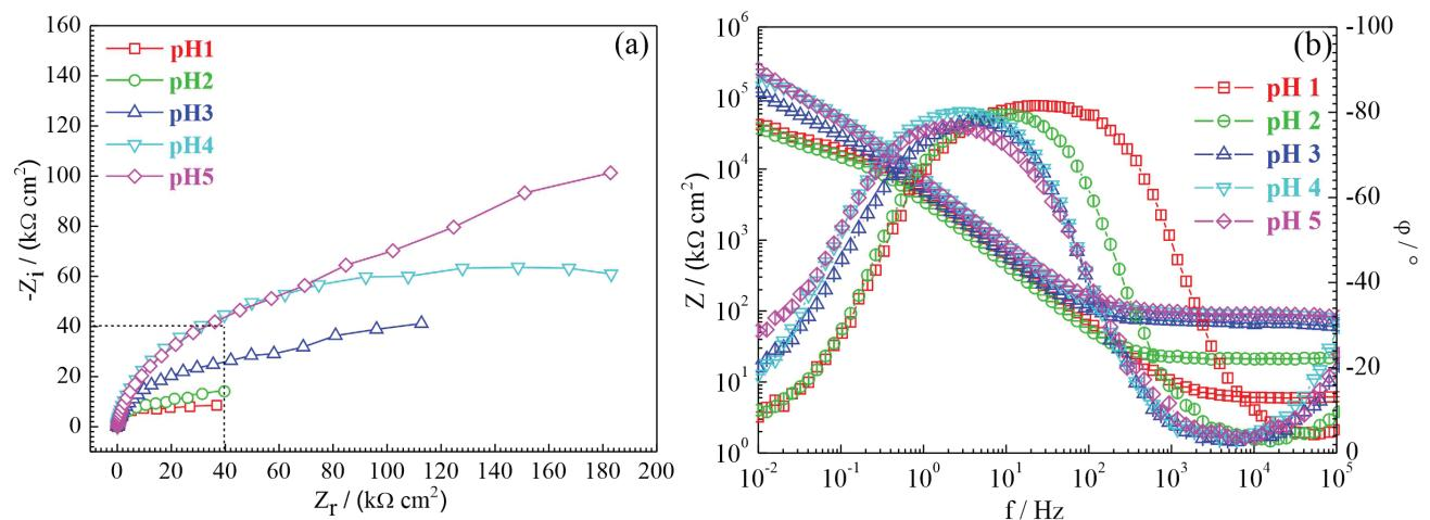
**Figure 7.** EIS of X65 samples in pH 1 to 5  $\text{HNO}_3$  solutions with  $0.01 \text{ mol L}^{-1} \text{NaNO}_2$  at the applied potential of  $1.0 \text{ V}_{\text{SCE}}$ : (a) Nyquist plot and (b) Bode plot.
