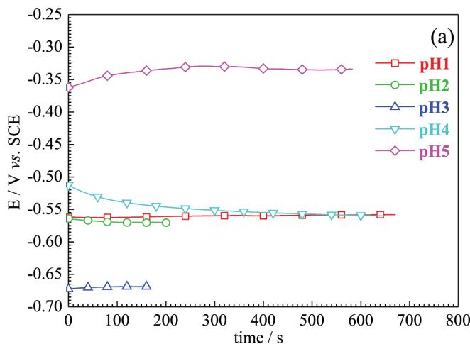
In the pH 1 to 3 solutions without NaNO<sub>2</sub>, with the raise of pH value, the E<sub>eq</sub> (H<sup>+</sup>/H<sub>2</sub>) value decreases, so the stable OCP and the E<sub>corr</sub> move to the negative direction.
