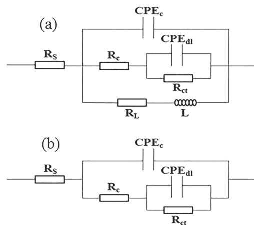
**Figure 6.** EEC model to fit EIS shown in Figure 5. (a) EIS obtained in the pH 1 to 3  $\text{HNO}_3$  solutions without  $\text{NaNO}_2$  and (b) EIS obtained in the pH 4 and 5  $\text{HNO}_3$  solutions without  $\text{NaNO}_2$  and in the pH 1 to 5  $\text{HNO}_3$  solutions with  $\text{NaNO}_2$ .
