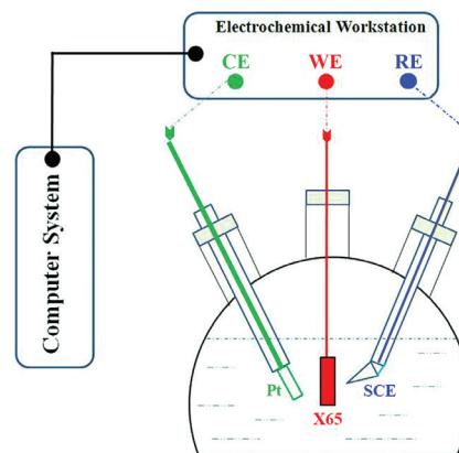
Figure 1. Schematic diagram of electrochemical testing system.
