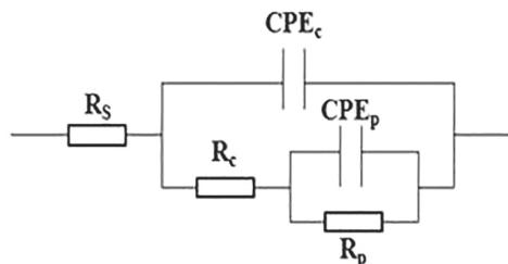
**Figure 8.** EEC model to fit EIS shown in Figure 7.
