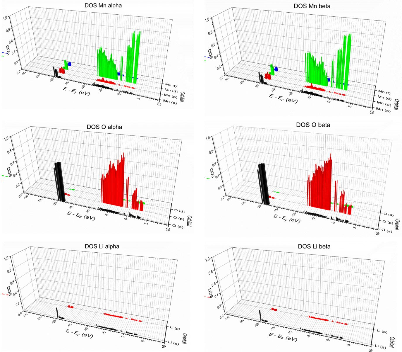
**Figure S7.** Density orbital state in optimized structure of  $\text{Li}_8\text{Mn}_{16}\text{O}_{32}$ . Method DFT/GGA, PBE-D3 functional, program CP2K, T (300 K).
