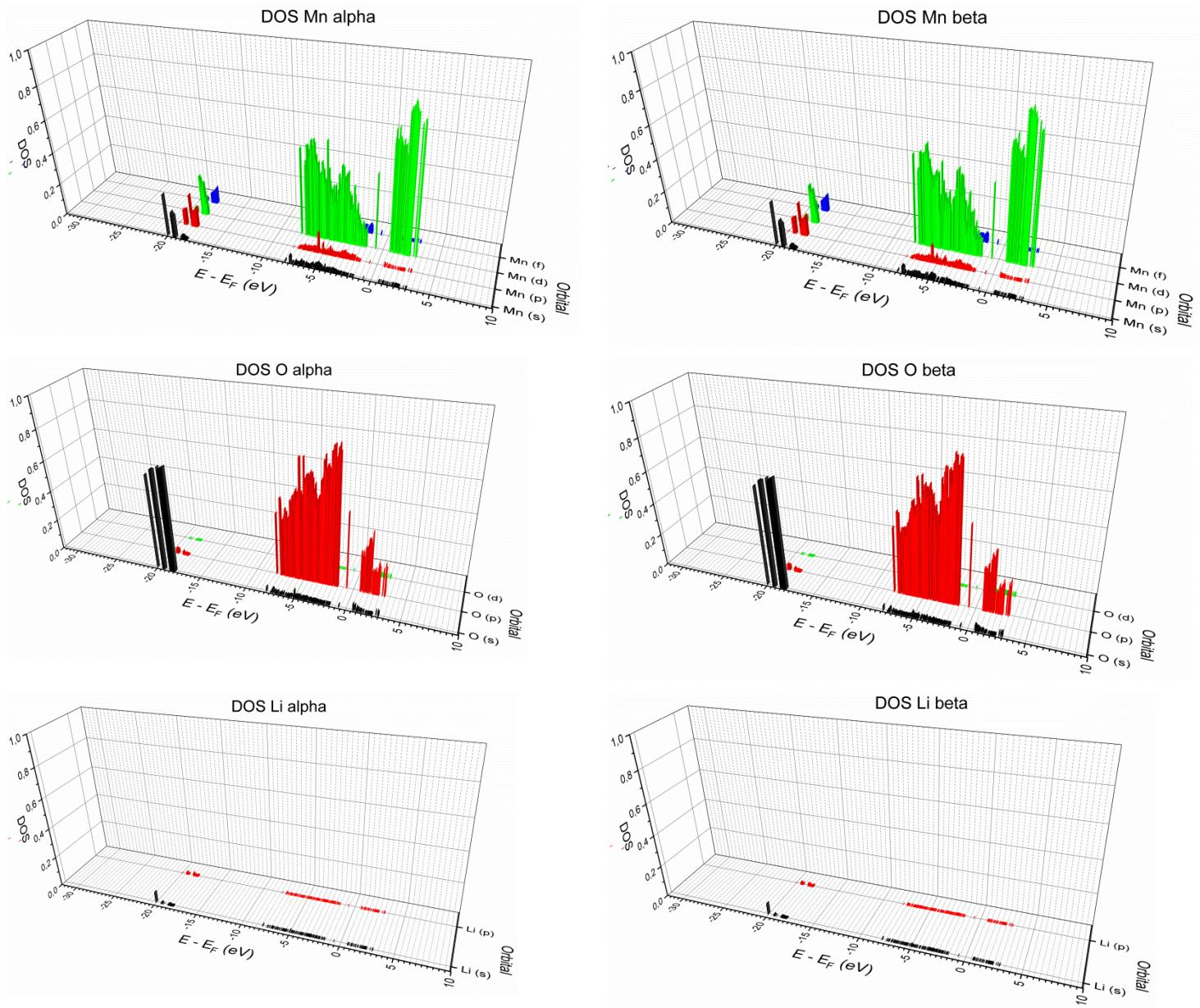
**Figure S3.** Density orbital state in optimized structure of  $\text{Li}_2\text{Mn}_{16}\text{O}_{32}$ . Method DFT/GGA, PBE-D3 functional, program CP2K, T (300 K).
