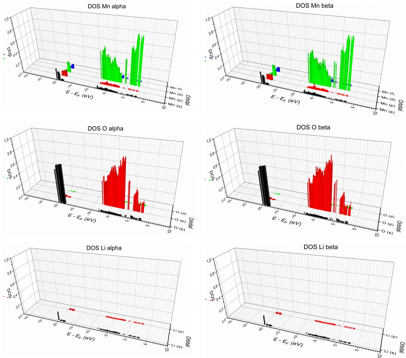
**Figure S5.** Density orbital state in optimized structure of  $\text{Li}_6\text{Mn}_{16}\text{O}_{32}$ . Method DFT/GGA, PBE-D3 functional, program CP2K, T (300 K).
