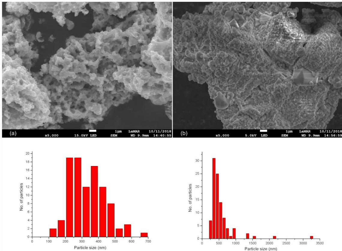
**Figure S10.** SEM images and histograms of LiMn<sub>2</sub>O<sub>4</sub> treated at: (a) 500 and (b) 700 °C.
