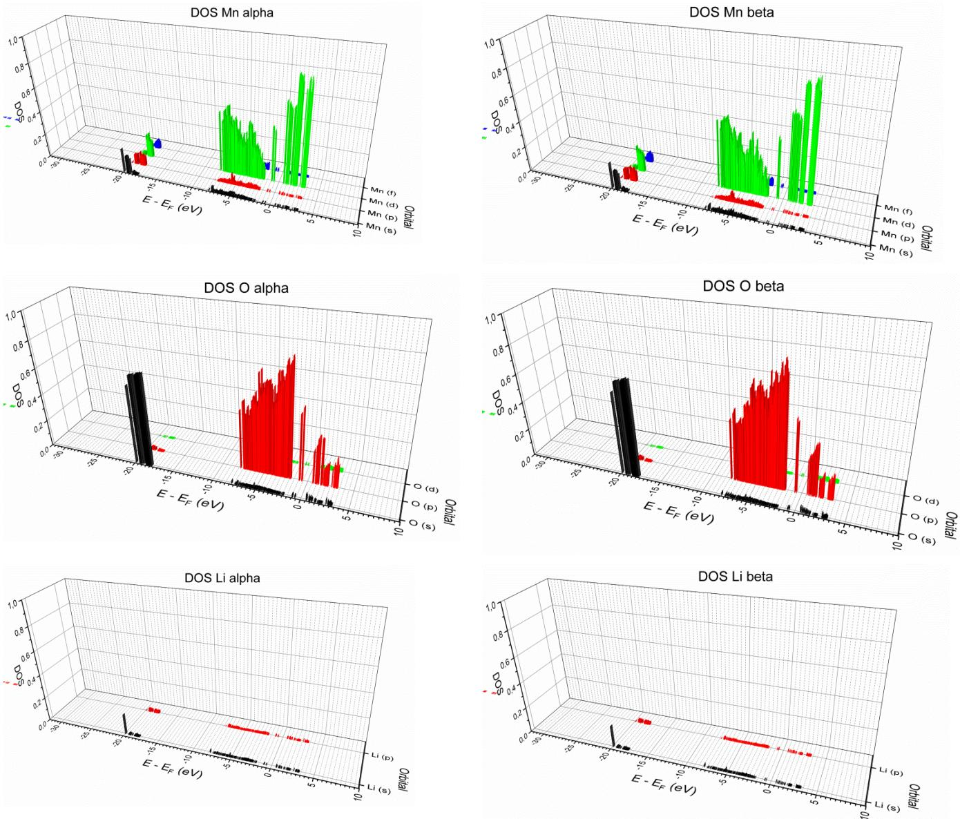
**Figure S6.** Density orbital state in optimized structure of  $\text{Li}_7\text{Mn}_{16}\text{O}_{32}$ . Method DFT/GGA, PBE-D3 functional, program CP2K, T (300 K).
