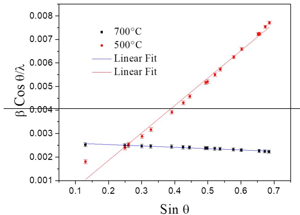
**Figure S1.** Williamson-Hall plotting to samples treated at 500 and 700 °C assuming the uniform deformation model.
