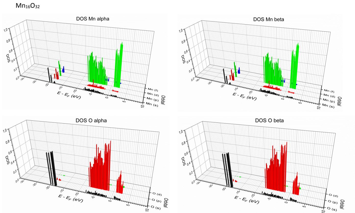
**Figure S2.** Density orbital state in optimized structure of  $\text{Mn}_{16}\text{O}_{32}$ . Method DFT/GGA, PBE-D3 functional, program CP2K, T (300 K).
