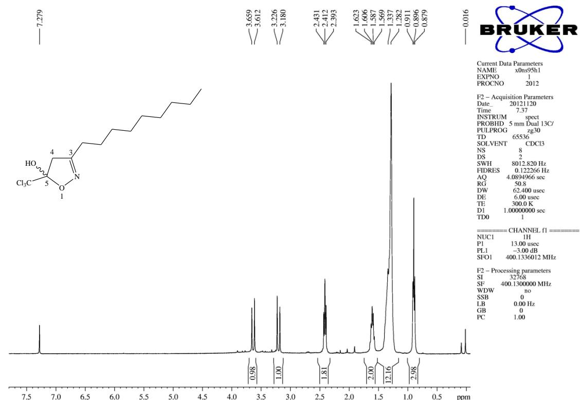
**Figure S105.** <sup>1</sup>H NMR spectrum (400 MHz, CDCl<sub>3</sub>) of 5-trichloromethyl-3-nonyl-5-hydroxy-4,5-dihydroisoxazole (**9c**).
