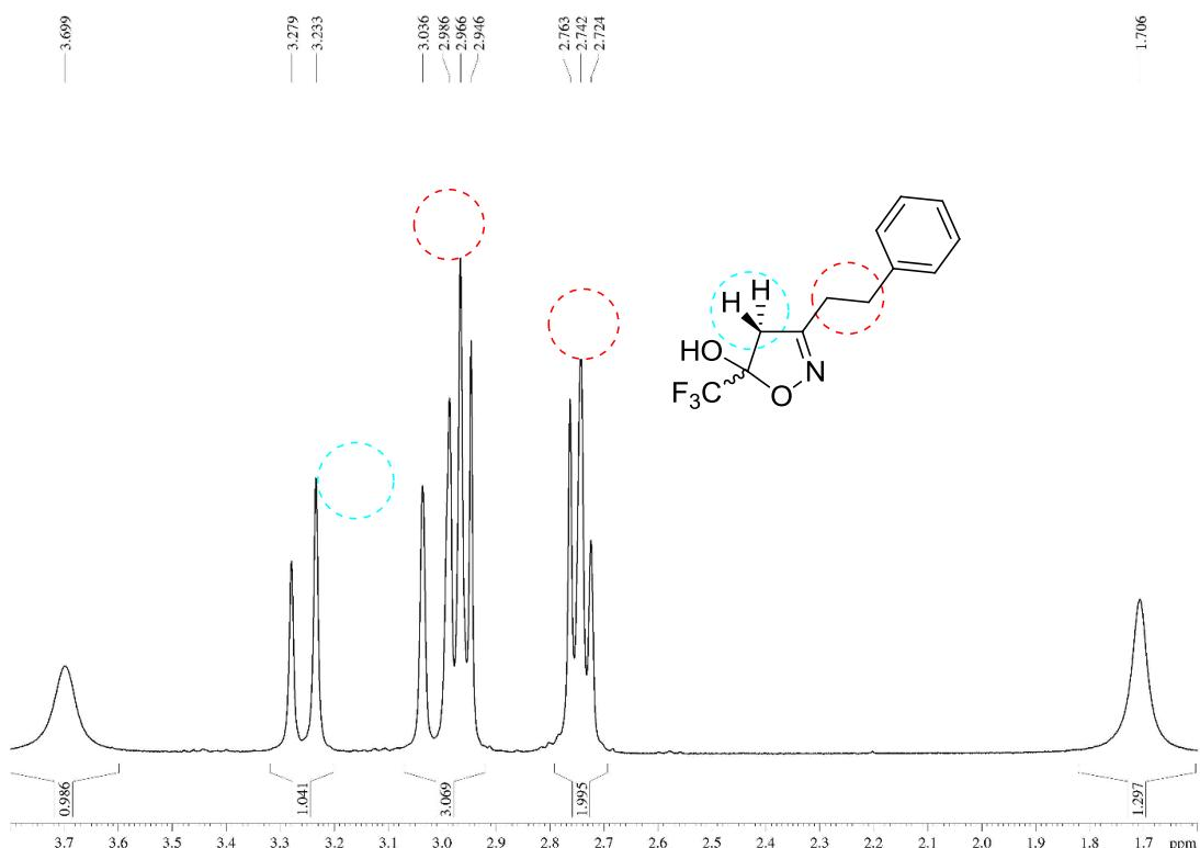
**Figure S79.** <sup>1</sup>H NMR spectrum (400 MHz, CDCl<sub>3</sub>) of the 5-hydroxy-3-phenethyl-5-(trifluoromethyl)-4,5-dihydroisoxazol (**8h**), expanded between 1.6-3.8 ppm.
