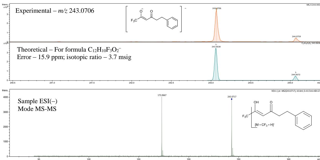
**Figure S70.** ESI MS-MS spectrum of the 1,1,1-trifluoro-4-methoxy-6-phenylhexan-2,4-dione (**5h**).
