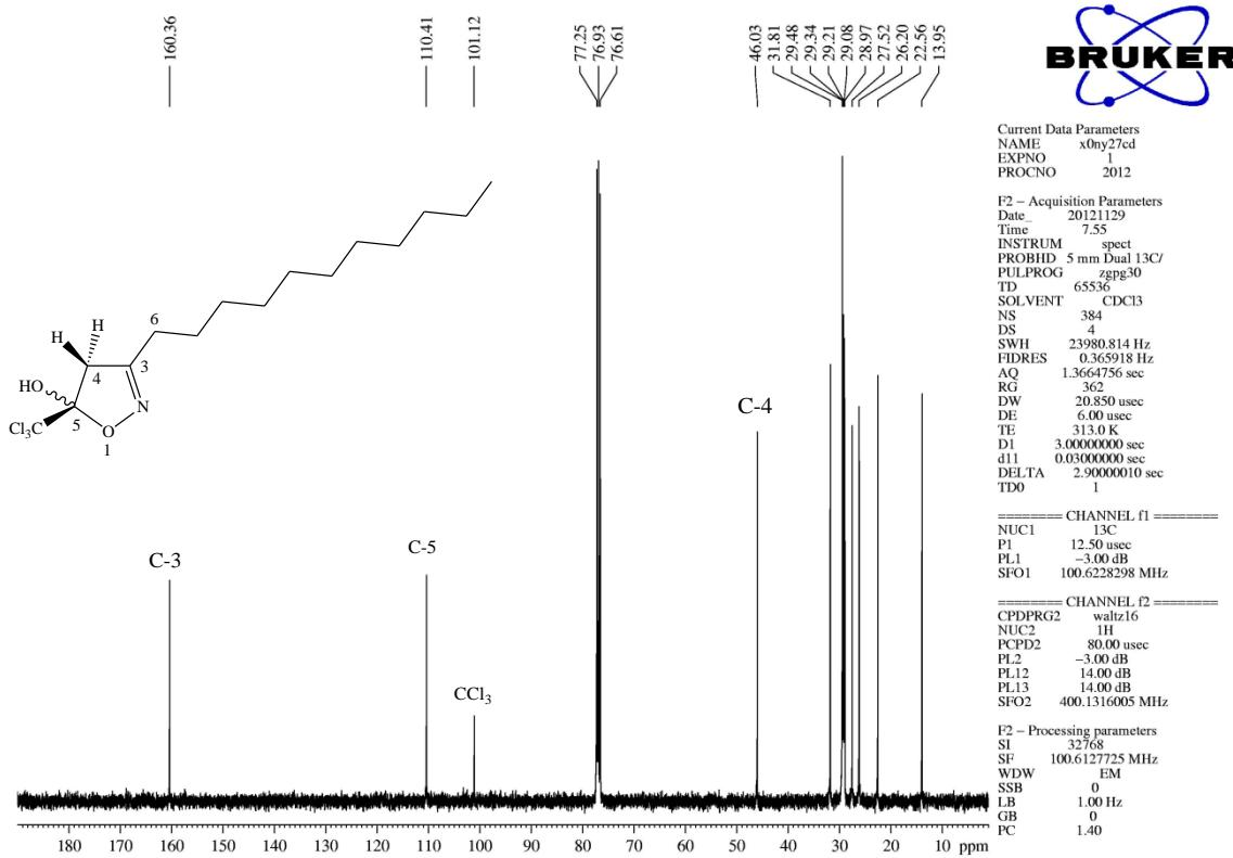
**Figure S108.**  $^{13}\text{C}$  NMR spectrum (400 MHz,  $\text{CDCl}_3$ ) of 5-trichloromethyl-3-undecyl-5-hydroxy-4,5-dihydroisoxazole (9e).
