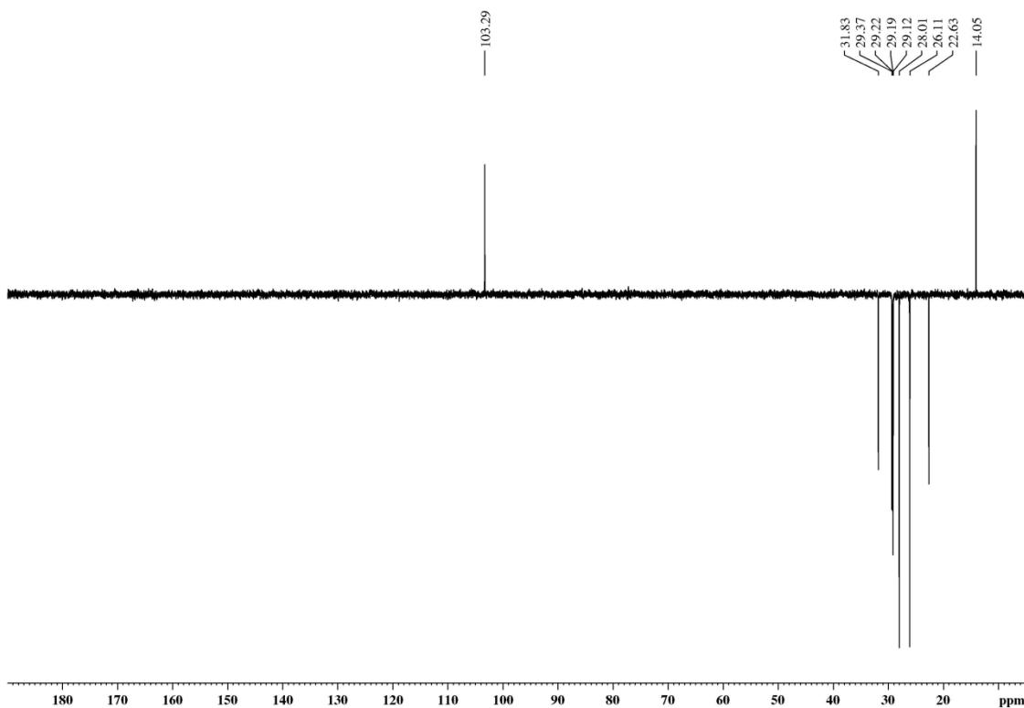
**Figure S120.**  $^{13}\text{C}$  DEPT135 NMR (400 MHz,  $\text{CDCl}_3$ ) spectrum of 5-trichloromethyl-3-nonylisoxazole (**11d**).
