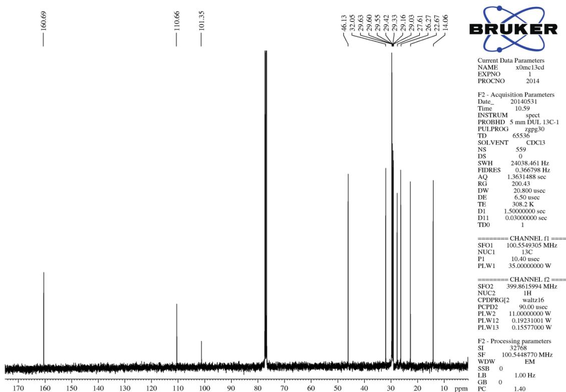
**Figure S111.**  $^{13}\text{C}$  NMR spectrum (400 MHz,  $\text{CDCl}_3$ ) of 5-trichloromethyl-3-tridecyl-5-hydroxy-4,5-dihydroisoxazole (**9f**).
