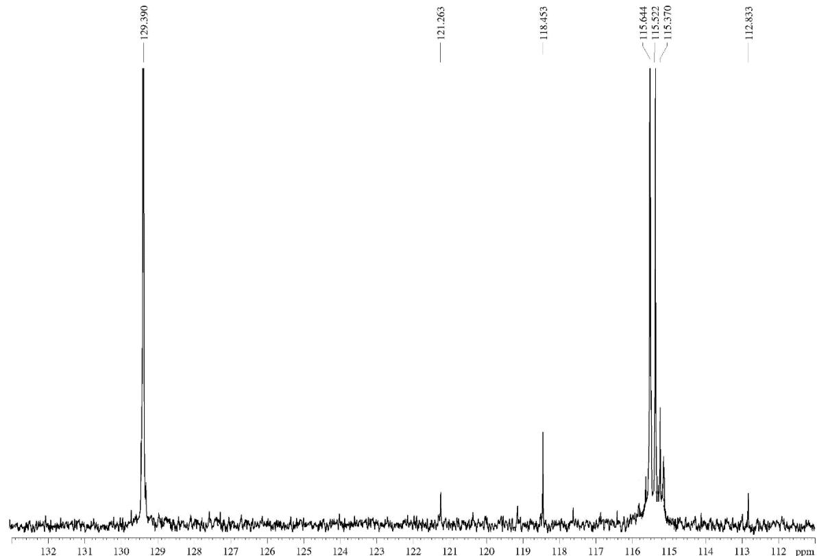
**Figure S73.**  $^{13}\text{C}$  NMR spectrum (100 MHz,  $\text{CDCl}_3$ ) of the 1,1,1-trifluoro-4-methoxy-6-(4-hydroxyphenyl)-hex-3-en-2-one (**5i**), expanded between 111-131 ppm.
