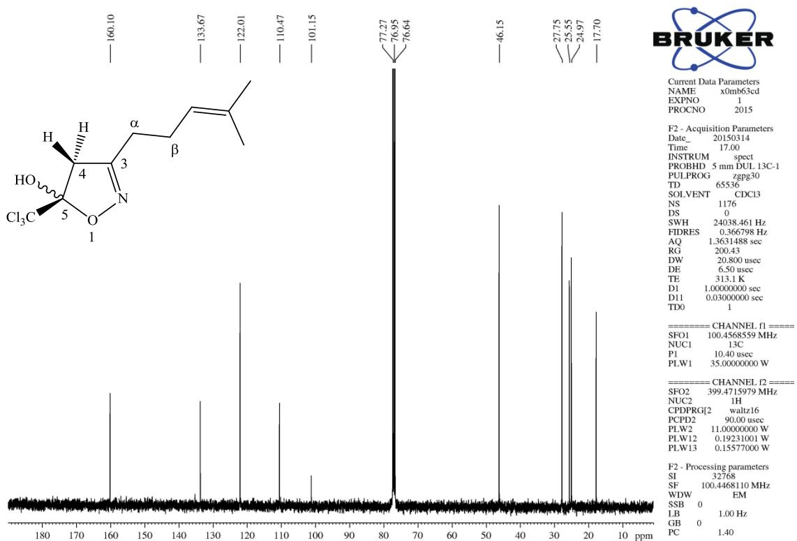
**Figure S114.** <sup>13</sup>C NMR spectrum (400MHz, CDCl<sub>3</sub>) of 5-trichloromethyl-3-(4-methyl-3-penten-1-yl)-5-hydroxy-4,5-dihydroisoxazole (**9g**).
