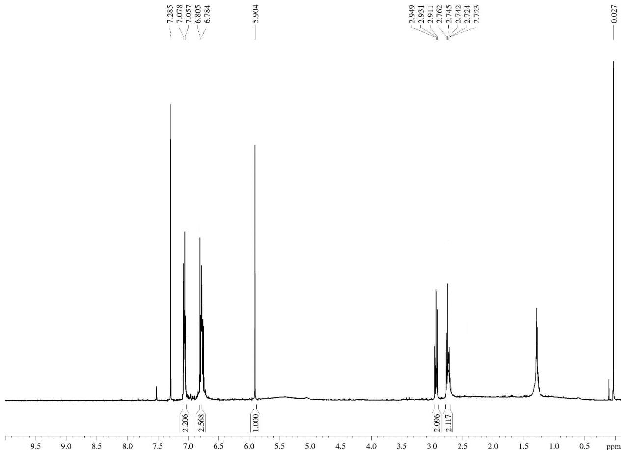
**Figure S71.**  $^1H$  NMR spectrum (400 MHz,  $CDCl_3$ ) of the 1,1,1-trifluoro-6-(4-hydroxyphenyl)-hexan-2,4-dione (**5i**).
