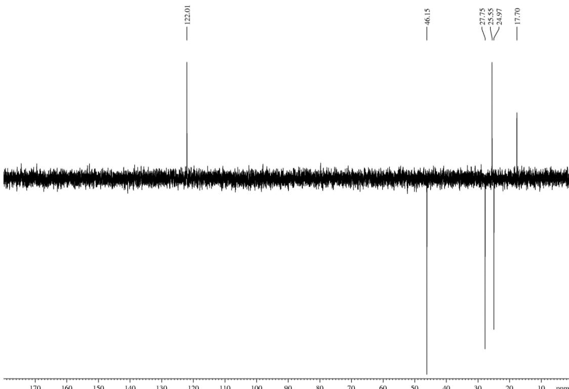
**Figure S115.** <sup>13</sup>C DEPT NMR spectrum (400MHz, CDCl<sub>3</sub>) of 5-trichloromethyl-3-(4-methyl-3-penten-1-yl)-5-hydroxy-4,5-dihydroisoxazole (**9g**).
