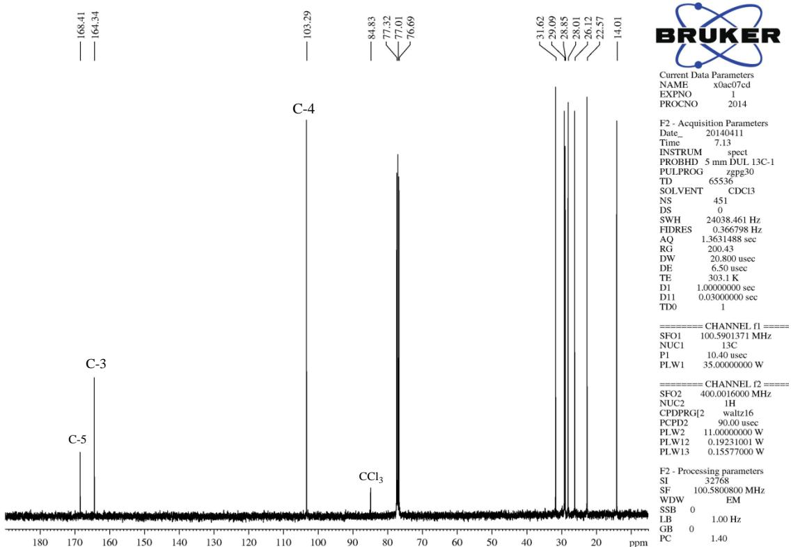
**Figure S117.**  $^{13}\text{C}$  NMR spectrum (400MHz, CDCl<sub>3</sub>) of 5-trichloromethyl-3-heptylisoxazole (**11a**).
