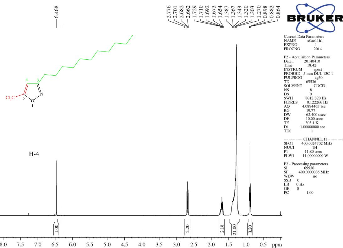
**Figure S121.**  $^1\text{H}$  NMR (400 MHz,  $\text{CDCl}_3$ ) spectrum of 5-trichloromethyl-3-undecylisoxazole (**11e**).
