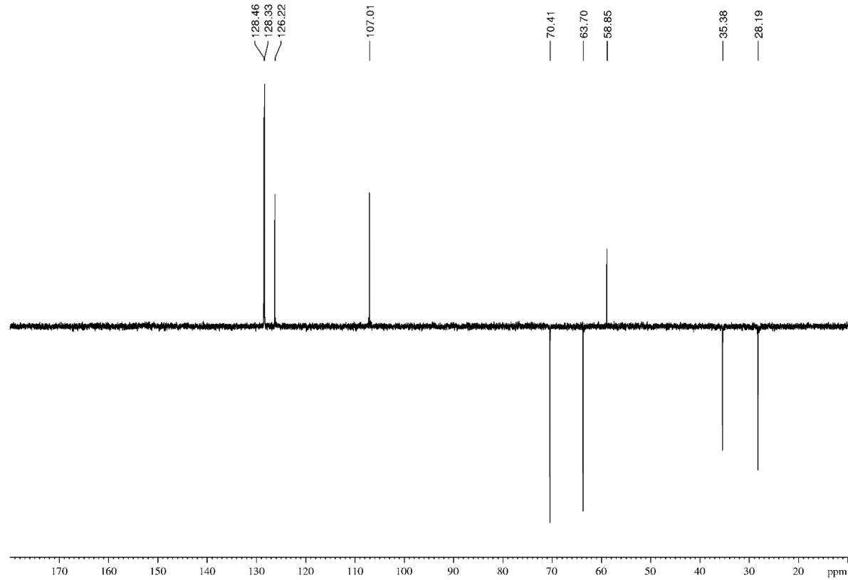
**Figure S100.** DEPT135  $^{13}\text{C}$  NMR spectrum (400 MHz,  $\text{CDCl}_3$ ) of 2-methoxyethyl 3-(2-phenylethyl)-1*H*-pyrazole-5-carboxylate (**14h**).
