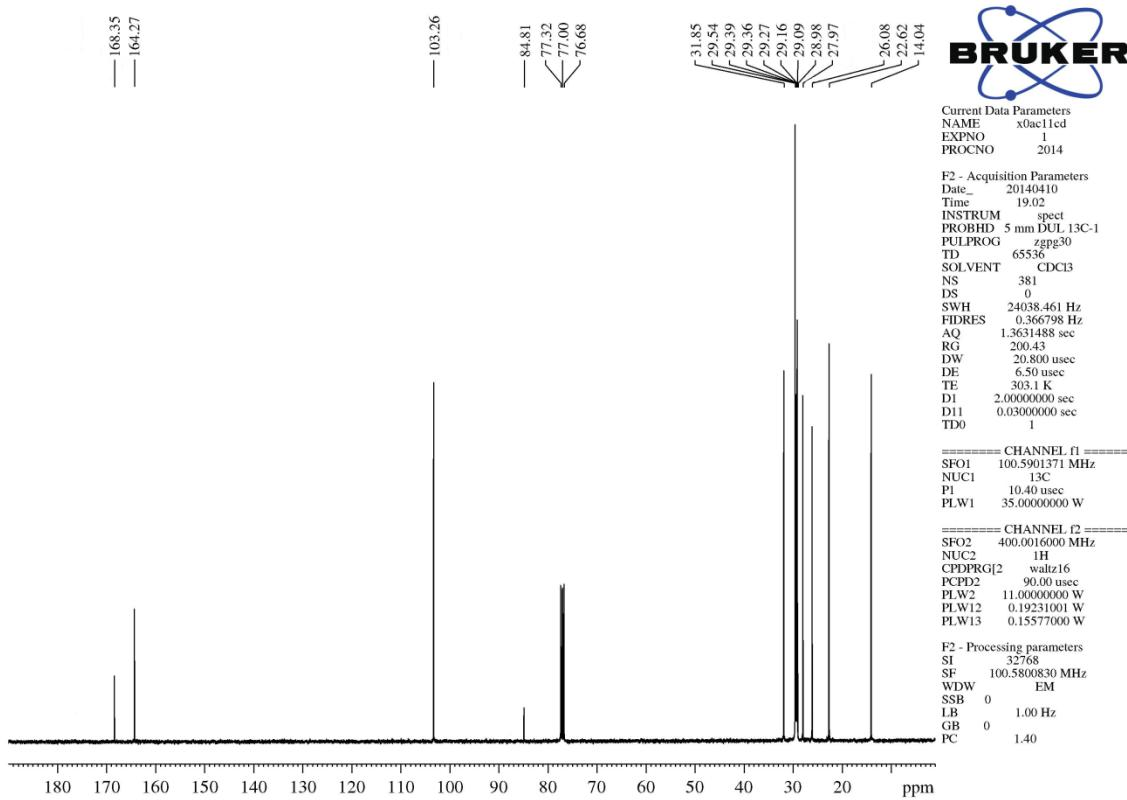
**Figure S122.** <sup>13</sup>C NMR (400 MHz, CDCl<sub>3</sub>) spectrum of 5-trichloromethyl-3-undecylisoxazole (**11e**).
