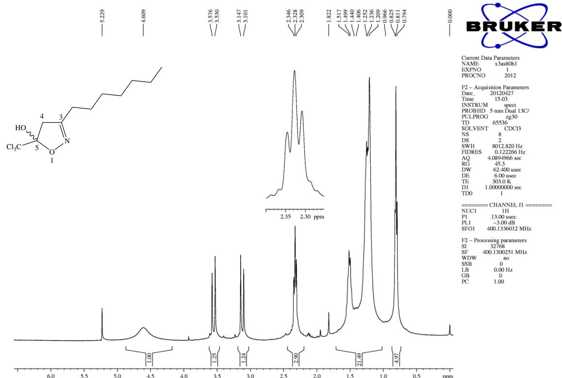
**Figure S101.**  $^1\text{H}$  NMR spectrum (400 MHz,  $\text{CDCl}_3$ ) of 5-trichloromethyl-3-heptyl-5-hydroxy-4,5-dihydroisoxazole (**9a**).
