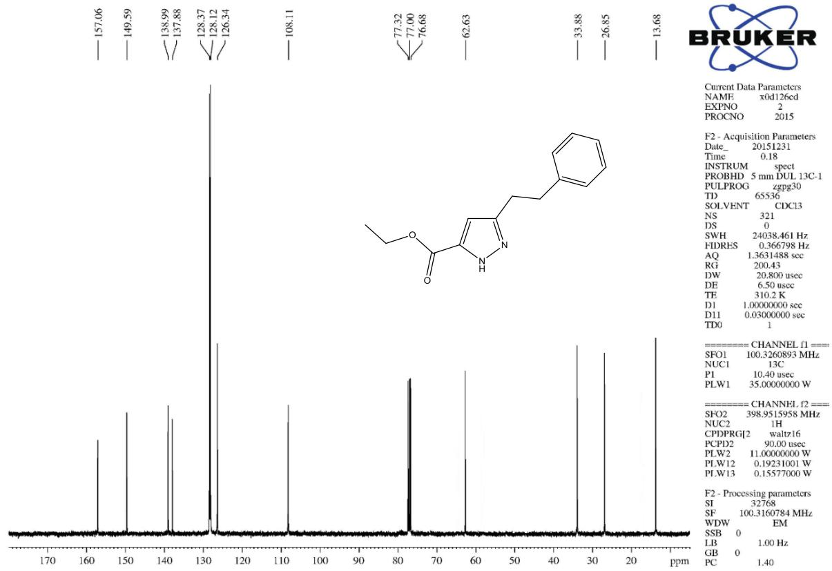
**Figure S96.**  $^{13}\text{C}$  NMR spectrum (400 MHz,  $\text{CDCl}_3$ ) of ethyl 3-(2-phenylethyl)-1*H*-pyrazole-5-carboxylate (**13h**).
