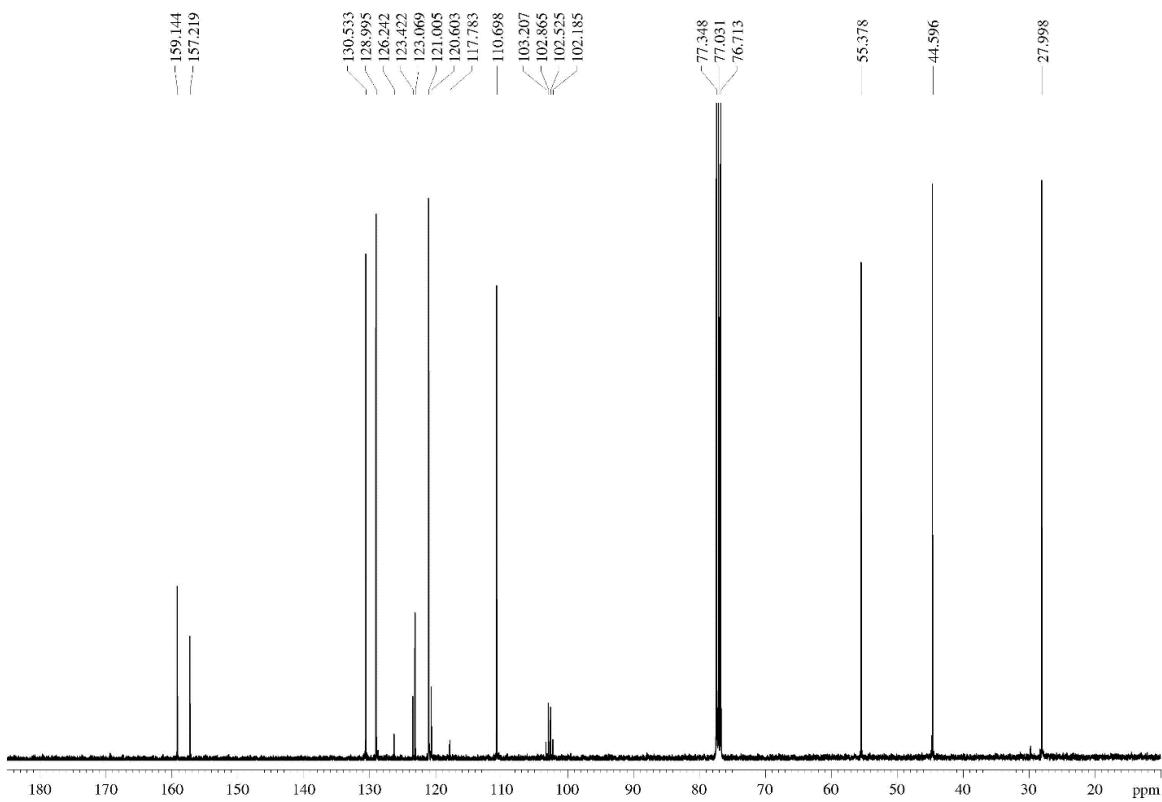
**Figure S86.**  $^{13}\text{C}$  NMR spectrum (100 MHz,  $\text{CDCl}_3$ ) of the 5-hydroxy-3-(2-methoxyphenyl)methyl-5-(trifluoromethyl)-4,5-dihydroisoxazole (**8I**).
