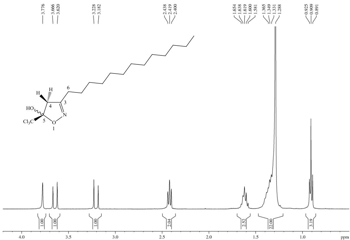
**Figure S110.**  $^1\text{H}$  NMR spectrum (400 MHz,  $\text{CDCl}_3$ ) of 5-trichloromethyl-3-tridecyl-5-hydroxy-4,5-dihydroisoxazole (**9f**), expanded between 0.6-4.2 ppm.
