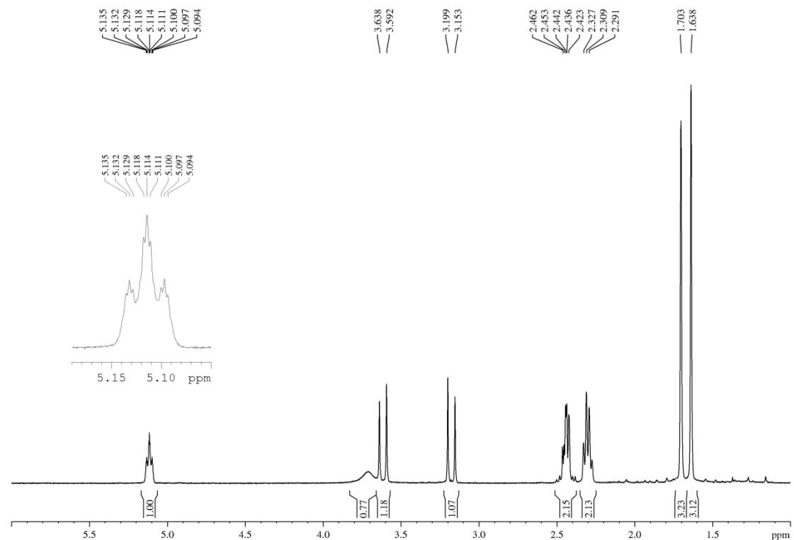
**Figure S113.**  $^1\text{H}$  NMR spectrum (400 MHz,  $\text{CDCl}_3$ ) of 5-trichloromethyl-3-(4-methyl-3-penten-1-yl)-5-hydroxy-4,5-dihydroisoxazole (**9g**), expanded between 1.0-6.0 ppm.
