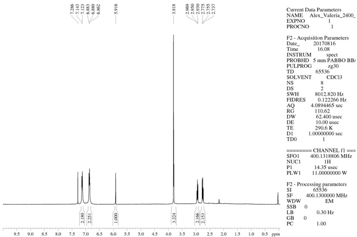
**Figure S74.** <sup>1</sup>H NMR spectrum (400 MHz, CDCl<sub>3</sub>) of the 1,1,1-trifluoro-6-(4-methoxyphenyl)hexan-2,4-dione (**5j**).
