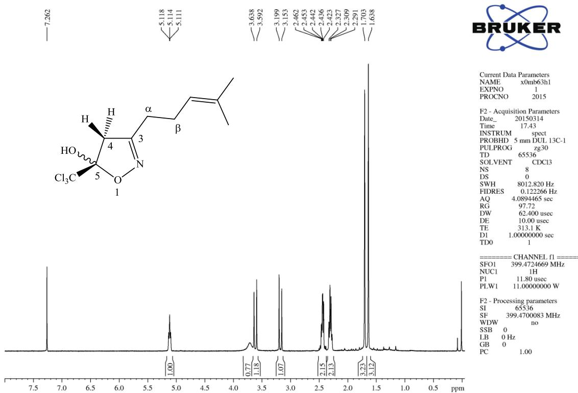
**Figure S112.**  $^1\text{H}$  NMR spectrum (400 MHz,  $\text{CDCl}_3$ ) of 5-trichloromethyl-3-(4-methyl-3-penten-1-yl)-5-hydroxy-4,5-dihydroisoxazole (**9g**).
