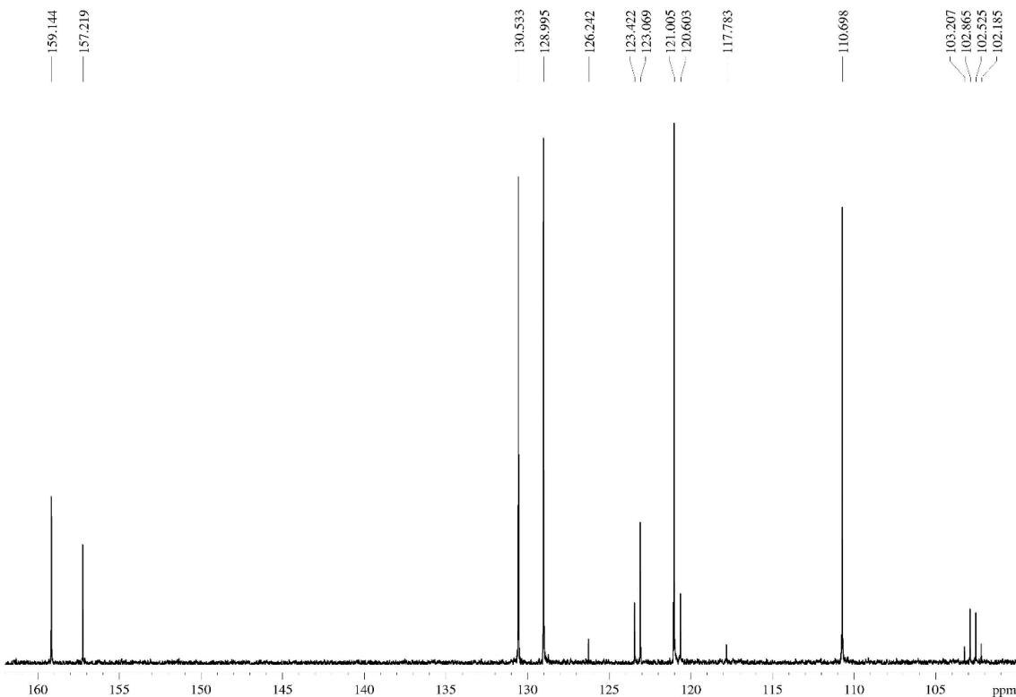
**Figure S87.**  $^{13}\text{C}$  NMR spectrum (100 MHz,  $\text{CDCl}_3$ ) of the 5-hydroxy-3-(2-methoxyphenyl)methyl-5-(trifluoromethyl)-4,5-dihydroisoxazole (**8I**), expanded between 100-162 ppm.
