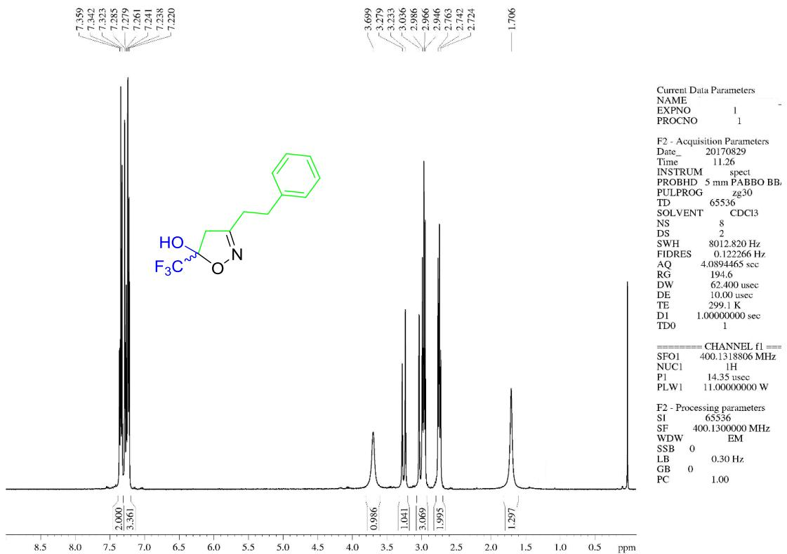
**Figure S78.** <sup>1</sup>H NMR spectrum (400 MHz, CDCl<sub>3</sub>) of the 5-hydroxy-3-phenethyl-5-(trifluoromethyl)-4,5-dihydroisoxazol (**8h**).
