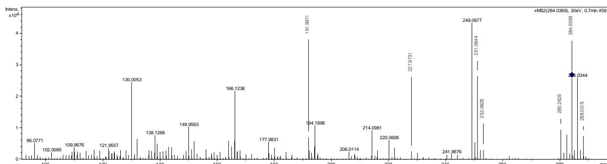
**Figure S129.** Mass spectra of 5-trichloromethyl-3-heptylisoxazole (**11a**).
