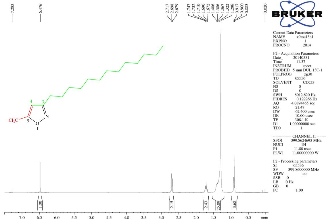
**Figure S123.** <sup>1</sup>H NMR (400 MHz, CDCl<sub>3</sub>) spectrum of 5-trichloromethyl-3-tridecylisoxazole (**11f**).
