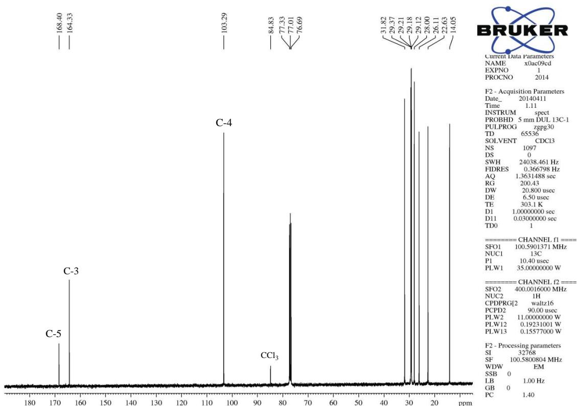
**Figure S119.**  $^{13}\text{C}$  NMR spectrum (400MHz,  $\text{CDCl}_3$ ) of 5-trichloromethyl-3-nonylisoxazole (**11d**).
