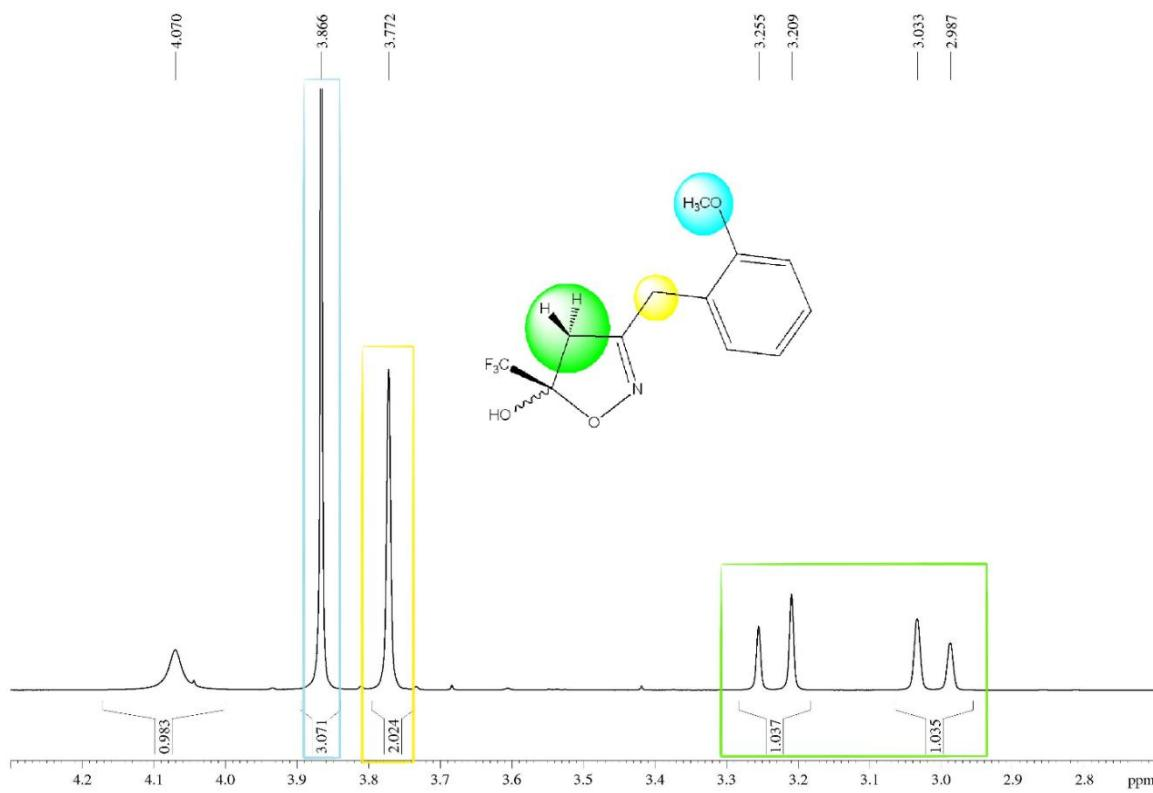
**Figure S84.**  $^1\text{H}$  NMR spectrum (400 MHz,  $\text{CDCl}_3$ ) of the 5-hydroxy-3-(2-methoxyphenyl)methyl-5-(trifluoromethyl)-4,5-dihydroisoxazole (**8I**), expanded between 2.7-4.3 ppm.
