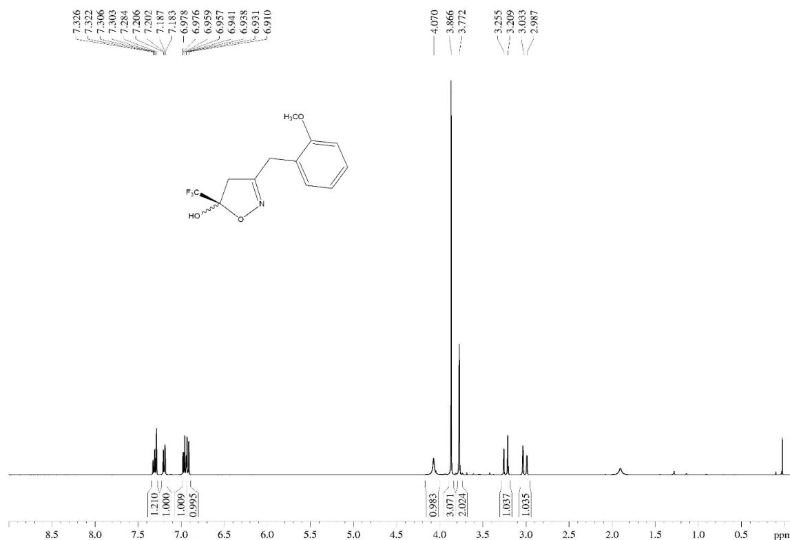
**Figure S83.**  $^1\text{H}$  NMR spectrum (400 MHz,  $\text{CDCl}_3$ ) of the 5-hydroxy-3-(2-methoxyphenyl)methyl-5-(trifluoromethyl)-4,5-dihydroisoxazole (**8I**).
