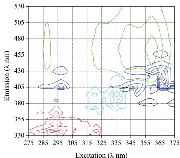
**Figure 2.** Contour plots for synthetic sample 15 (see Table 1). BaP (blue); ACL (red); PYR (cyan); ANT (black); PHN (magenta) and FLT (green).
