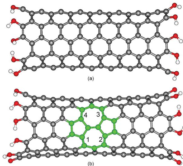
**Figure 1.** Molecular models for an SWCNT with the molecular formula  $\text{C}_{180}\text{H}_{22}\text{O}_{22}$ : (a) pristine (P) and (b) Stone-Wales (SW) defect in green. The carbon atoms indicated by positions 1-4 were substituted by oxygen atoms to create the models named SW-1O, SW-2O, SW-3O and SW-4O.
