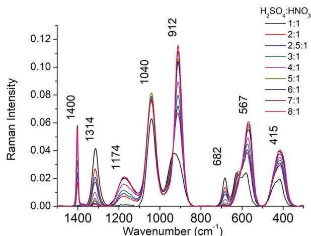
**Figure 3.** Raman spectra of acid mixtures in different  $\text{H}_2\text{SO}_4:\text{HNO}_3$  proportions (v/v): 1:1, 2:1, 2.5:1, 3:1, 4:1, 5:1, 6:1, 7:1 and 8:1.
