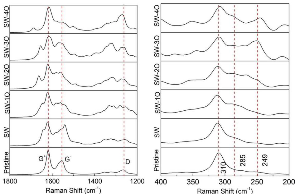
**Figure 8.** Simulated Raman spectra for the proposed models in the (a) 1800-1200 cm<sup>-1</sup> region and (b) RBM region, 400-200 cm<sup>-1</sup>.
