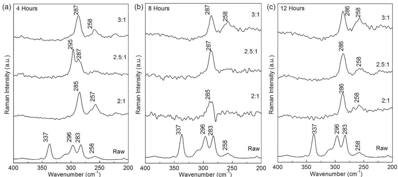
**Figure 5.** Raman spectra in the range of  $200\text{--}400\text{ cm}^{-1}$  for the oxidized samples for (a) 4 h, (b) 8 h and (c) 12 h of reaction. The bands are assigned to RBMs.
