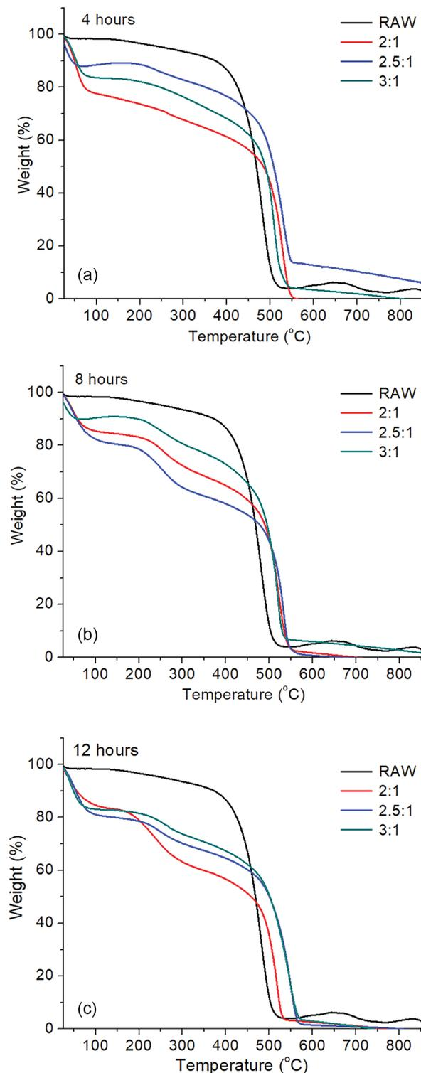
**Figure 6.** Thermogram of the oxidized samples for (a) 4 h, (b) 8 h and (c) 12 h of oxidation.
