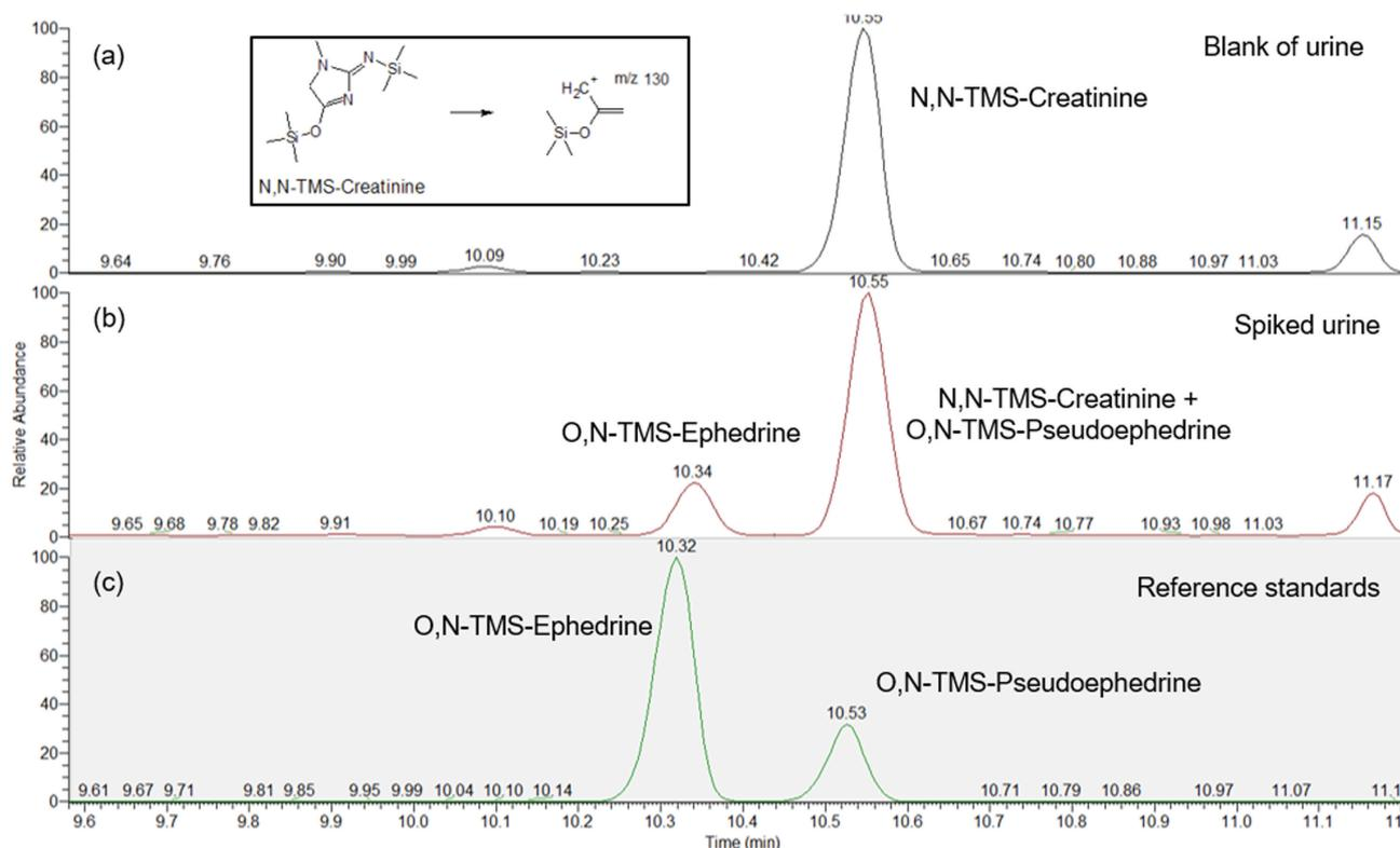
**Figure 1.** Comparison of (a) blank urine; (b) urine spiked with ephedrines at the respective threshold and (c) reference standards chromatograms regarding the  $m/z$  130 detection after MSTFA reaction.
