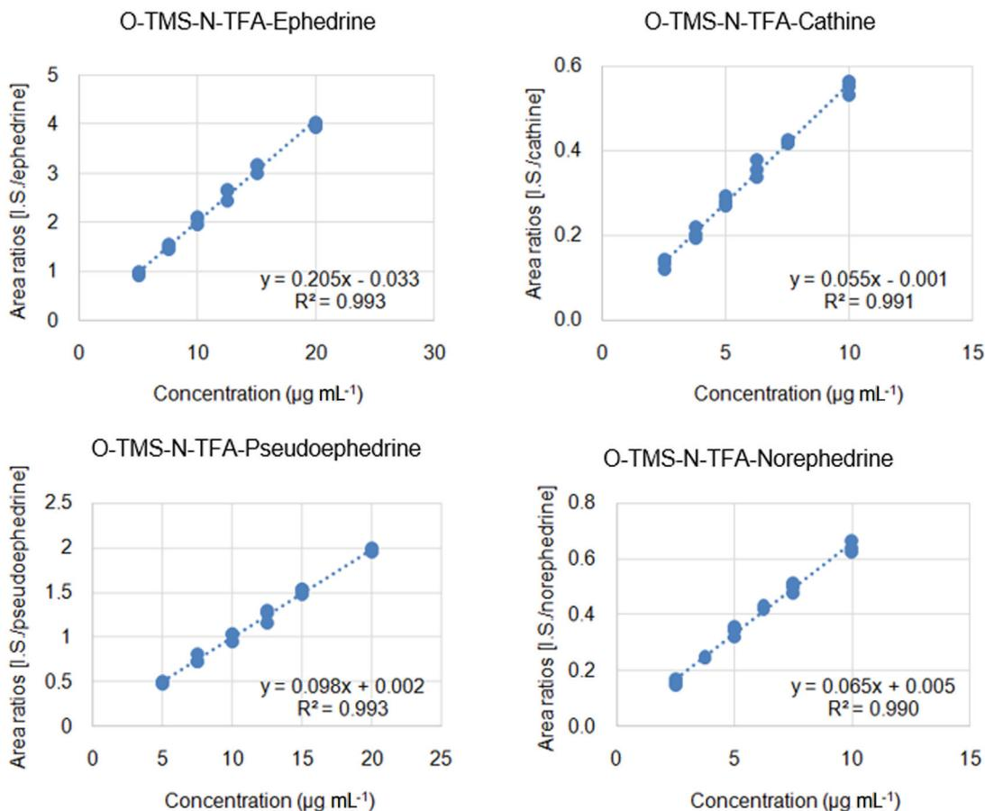
**Figure 5.** Calibration curves for the linearity evaluation for ephedrine-O-TMS-N-TFA, O-TMS-N-TFA-cathine, O-TMS-N-TFA-pseudoephedrine and O-TMS-N-TFA-norephedrine.
