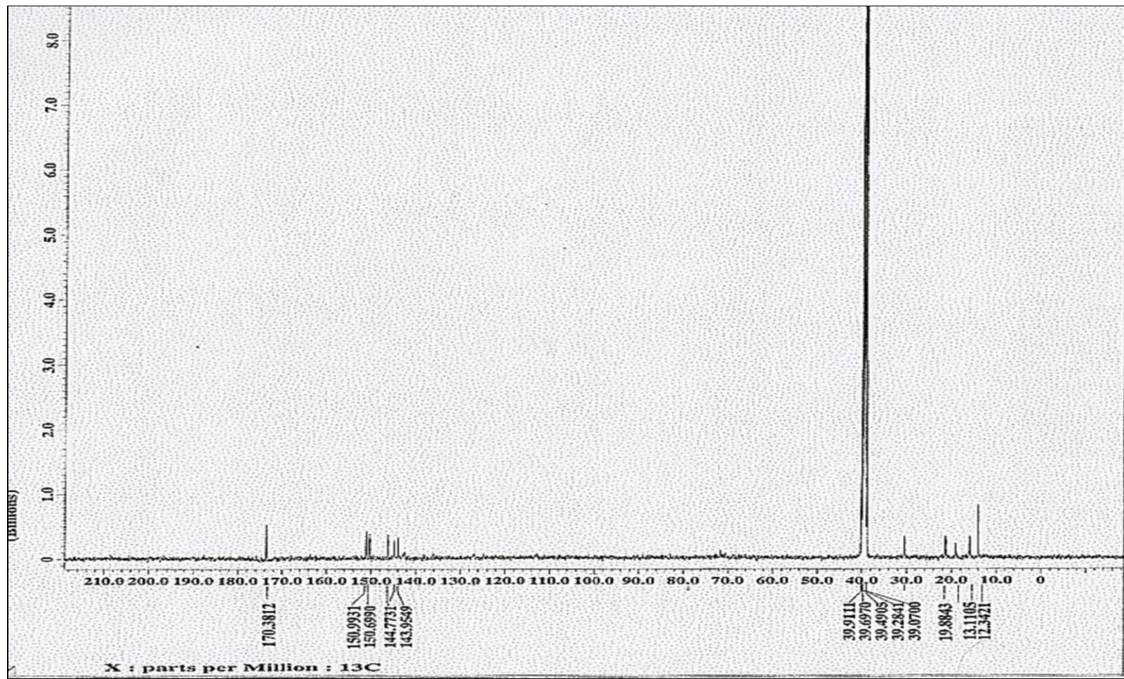
Figure S5.  $^{13}\text{C}$  NMR (400 MHz,  $\text{DMSO}-d_6$ ) spectrum of APBT.
