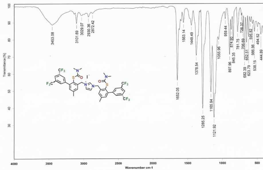
**Figure S8.** IR (KBr) spectrum of **3**.
