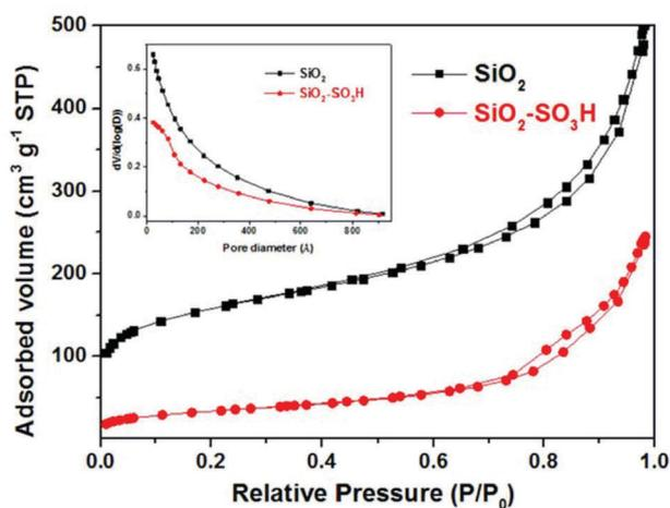
Figure 5.  $\text{N}_2$  adsorption/desorption isotherms and (inset) Barrett-Joyner-Halenda (BJH) method to pore size distributions for pure silica ( $\text{SiO}_2$ ) (black squares) before modifications and  $\text{SiO}_2\text{-SO}_3\text{H}$  (red squares).
