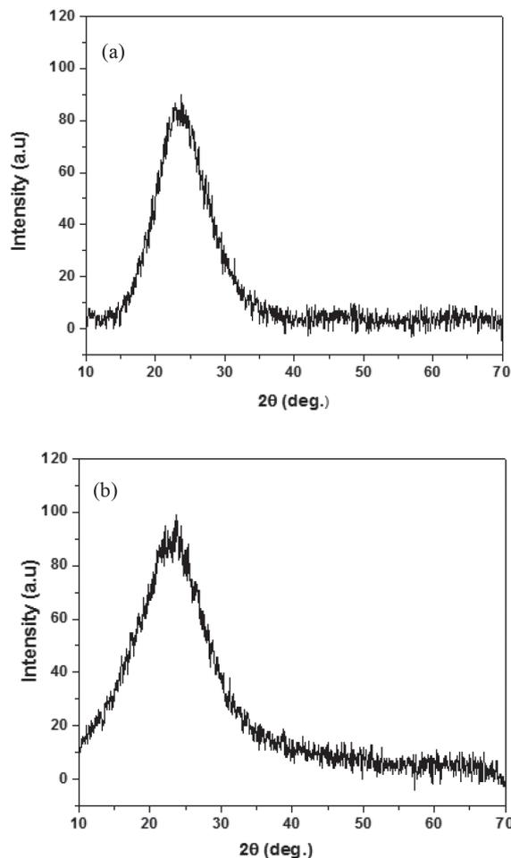
**Figure 1.** X-ray powder pattern of (a) precipitated silica gel and (b) SiO<sub>2</sub>-SO<sub>3</sub>H catalyst.
