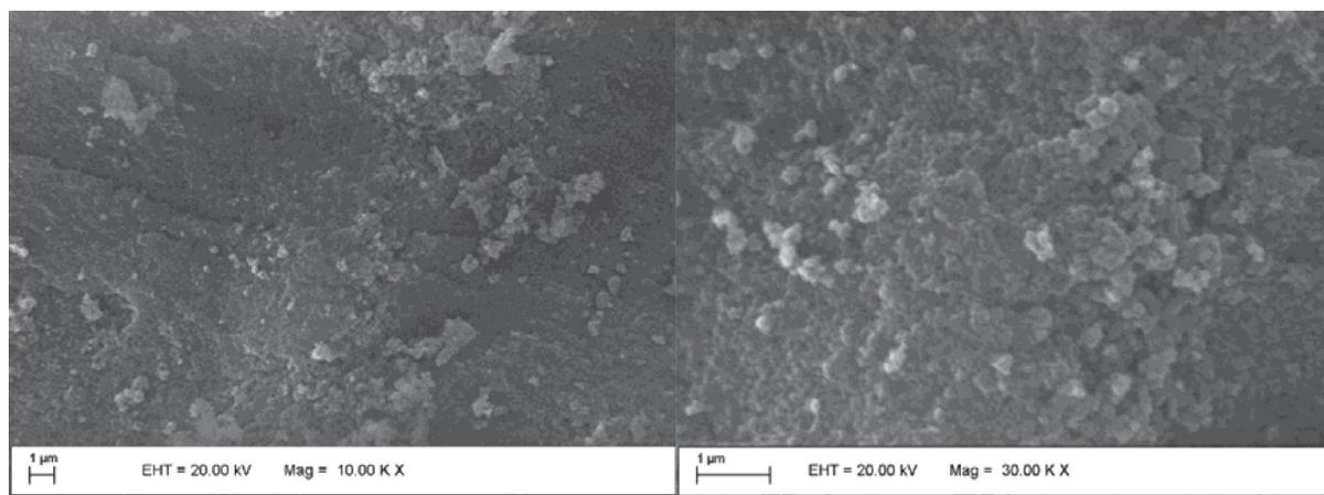
Figure 3. FE-SEM images of the amorphous silica gel.
