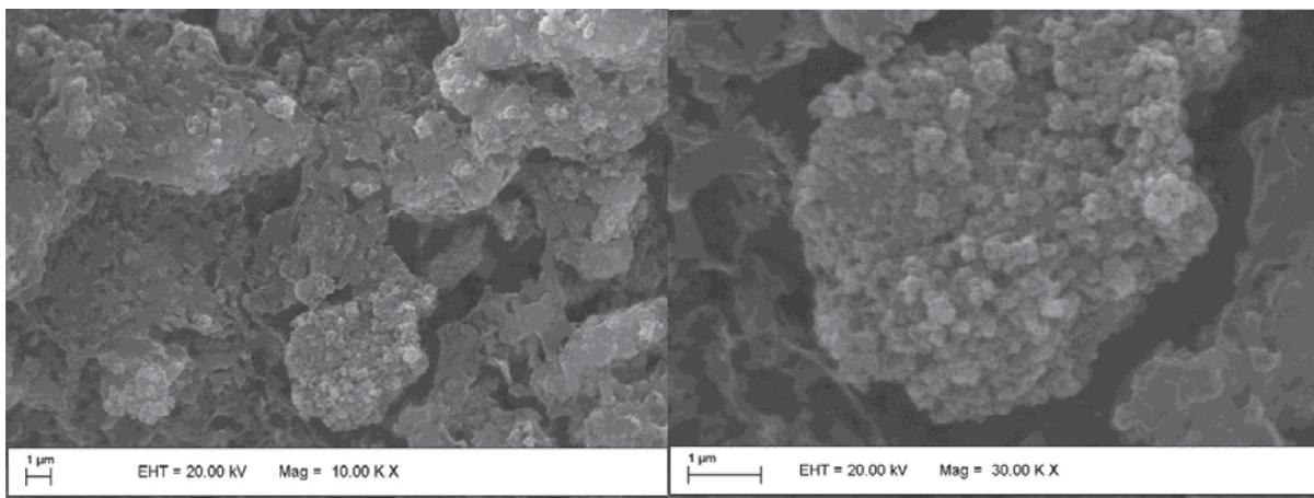
Figure 4. FE-SEM images of the  $\text{SiO}_2\text{-SO}_3\text{H}$ .
