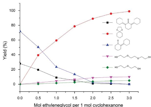
**Figure 7.** Product distribution of the reaction of 1 mol equiv. of cyclohexanone to 0-3 mol equiv. ethylene glycol, 10% (m/m) of catalyst to ketone; 2 min MW irradiation at 360 W; final temperature ca. 70 °C.
