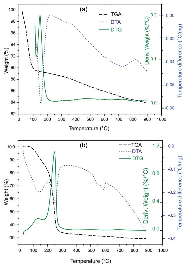
Figure 6. TGA/DTG/DTA curves of (a) new silica gel and (b) catalyst in a synthetic air atmosphere (25 to  $900^\circ\text{C}$ ).
