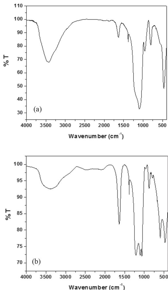
Figure 2. FTIR spectra of the (a) silica gel and (b)  $\text{SiO}_2\text{-SO}_3\text{H}$ .
