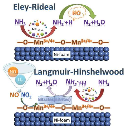
**Figure 10.** NO removal mechanism of the Mn<sub>7.5</sub>/FMN catalyst.
