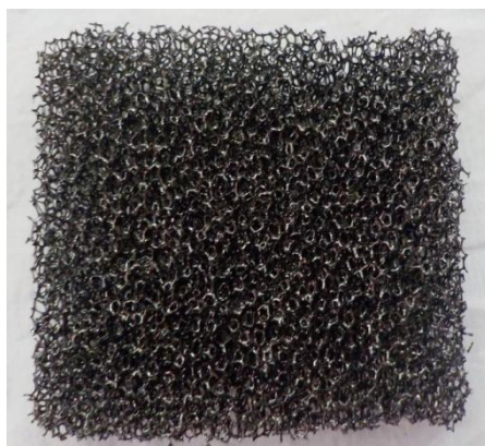
Figure S1. RVC substrate (45 ppi, 0.5 × 2.5 × 2.5 cm).
