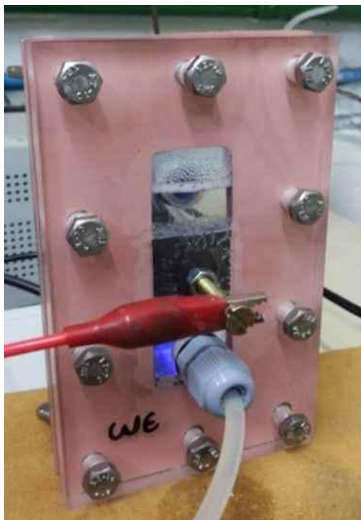
Figure S4. Photograph of the electrochemical reactor.
