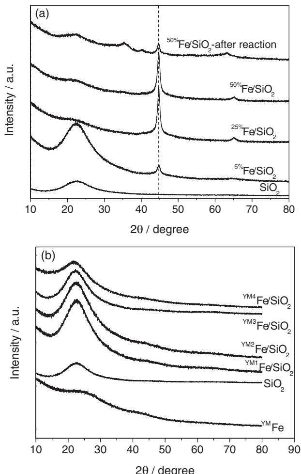
**Figure 1.** X-Ray diffraction (XRD) patterns of the  $\text{Fe/SiO}_2$  catalysts. (a) Prepared with  $\text{NaBH}_4$ ; and (b) prepared with yerba mate tea extract.
