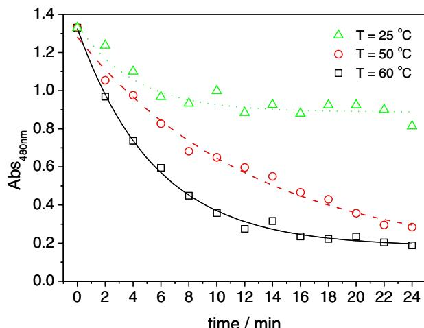
**Figure 12.** Time trace of methyl orange degradation ( $5.0 \times 10^{-5}$  mol L $^{-1}$ ) with  $^{YM_3}\text{Fe}/\text{SiO}_2$  at pH 5.0 at different temperatures (T).
