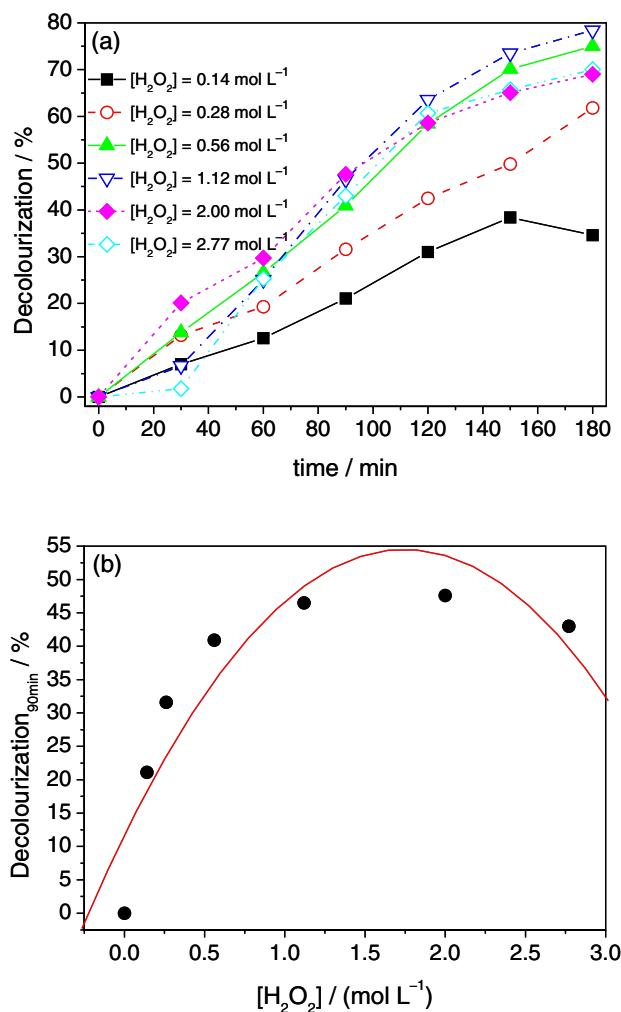
**Figure 10.** Decolorization of methyl orange ( $5.0 \times 10^{-5} \text{ mol L}^{-1}$ ) at different concentrations of  $\text{H}_2\text{O}_2$  using 40 mg of  ${}^{\text{YM}2}\text{Fe}/\text{SiO}_2$  at 25 °C and pH 3.5. (a) Decolorization vs. reaction time; and (b) decolorization at 90 min vs.  $\text{H}_2\text{O}_2$  concentration ( $[\text{H}_2\text{O}_2]$ ).
