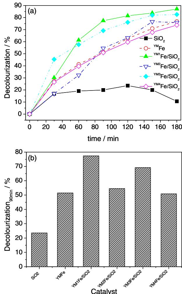
**Figure 13.** Decolourization of methyl orange ( $5.0 \times 10^{-5}$  mol L $^{-1}$ ) with different catalysts (60 mg) and  $\text{H}_2\text{O}_2$  (0.56 mol L $^{-1}$ ) at 25 °C and pH 3.5. (a) Decolourization vs. reaction time; and (b) decolourization at 90 min vs. catalyst.
