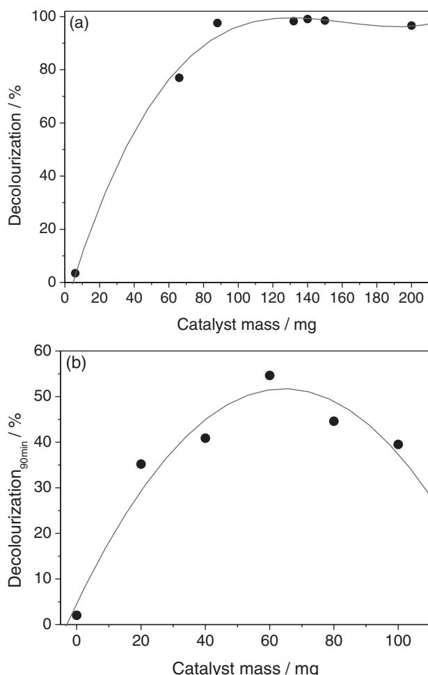
**Figure 8.** Maximum decolorization of methyl orange ( $5.0 \times 10^{-5}$  mol L $^{-1}$ ) vs. catalyst mass, at 25 °C, pH 5.0, catalyzed by (a)  $^{50\%}\text{Fe}/\text{SiO}_2$ ; and (b)  $^{YM2}\text{Fe}/\text{SiO}_2$ , H $_2$ O $_2$  (0.56 mol L $^{-1}$ ).
