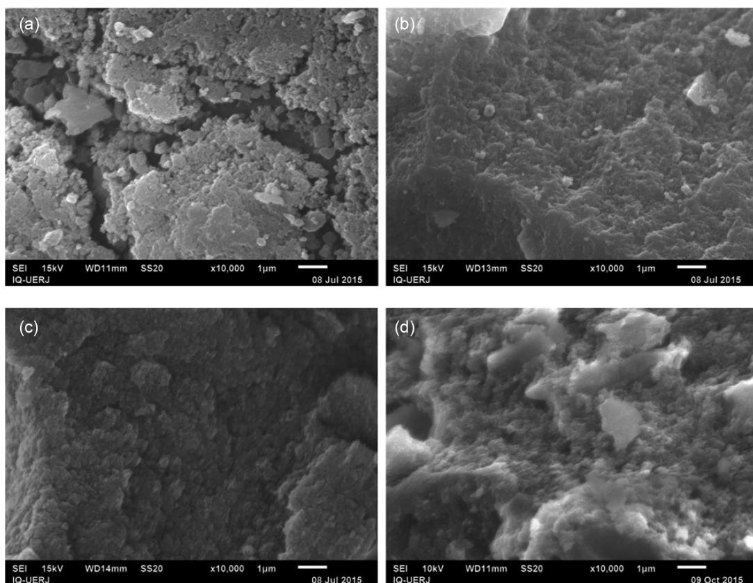
**Figure 3.** Scanning electron microscopy (SEM) micrographs of the catalysts (10,000 $\times$ ). (a)  $^{YM1}$ Fe/SiO<sub>2</sub>; (b)  $^{YM2}$ Fe/SiO<sub>2</sub>; (c)  $^{YM3}$ Fe/SiO<sub>2</sub>; and (d)  $^{YM4}$ Fe/SiO<sub>2</sub>.
