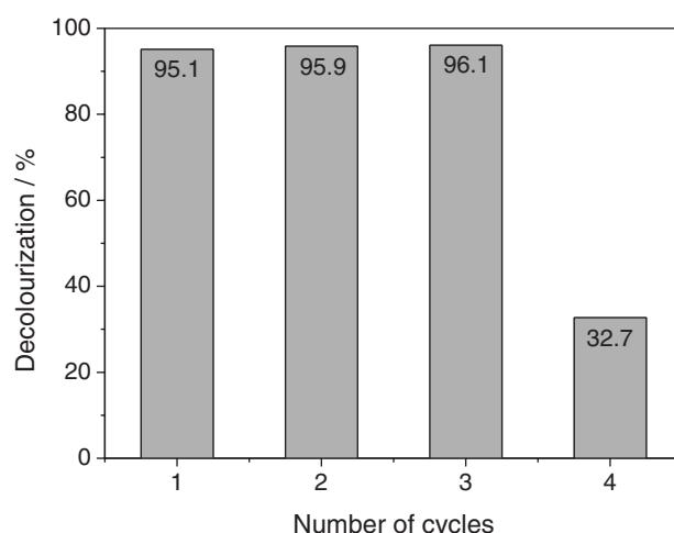
**Figure 9.** Recycle of the  $^{50\%}\text{Fe}/\text{SiO}_2$  catalyst (40 mg) in methyl orange ( $5.0 \times 10^{-5}$  mol L $^{-1}$ , 30 mL) degradation at 25 °C, pH 5.0.
