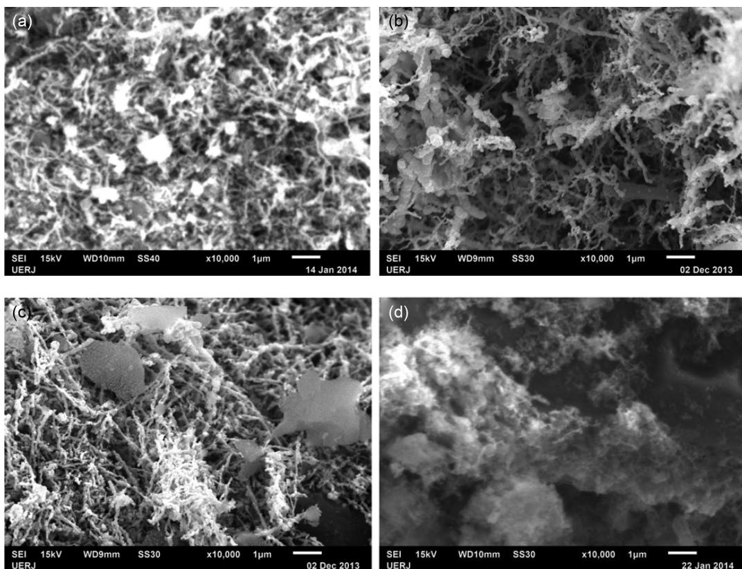
**Figure 2.** Scanning electron microscopy (SEM) micrographs of the catalysts (10,000 $\times$ ). (a)  $50\%$ Fe/SiO<sub>2</sub>; (b)  $25\%$ Fe/SiO<sub>2</sub>; (c)  $5\%$ Fe/SiO<sub>2</sub>; (d)  $50\%$ Fe/SiO<sub>2</sub> after reaction.
