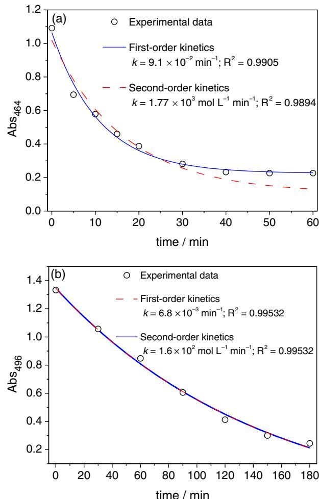
**Figure 7.** Kinetics first and second order fits of the time trace of methyl orange degradation ( $5.0 \times 10^{-5}$  mol L<sup>-1</sup>) at 25 °C and pH 5.0, with (a) <sup>50%</sup>Fe/SiO<sub>2</sub> (132.0 mg); and (b) <sup>YM2</sup>Fe/SiO<sub>2</sub> (40.0 mg), H<sub>2</sub>O<sub>2</sub> (0.56 mol L<sup>-1</sup>).
