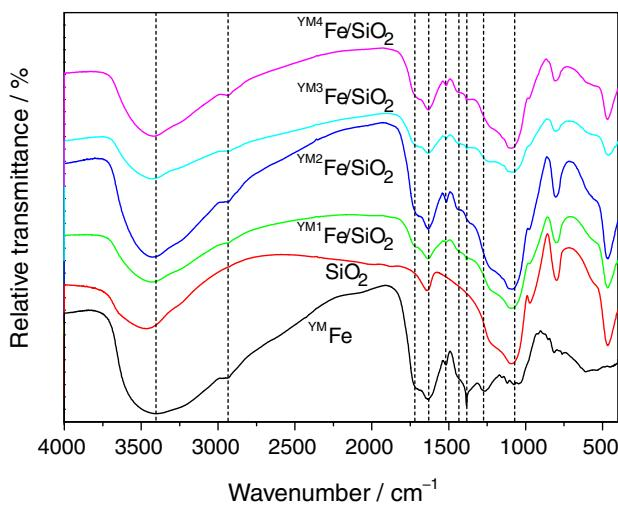
**Figure 4.** Fourier transform infrared (FTIR) spectra of the Fe/SiO<sub>2</sub> catalysts prepared with yerba mate tea extract.
