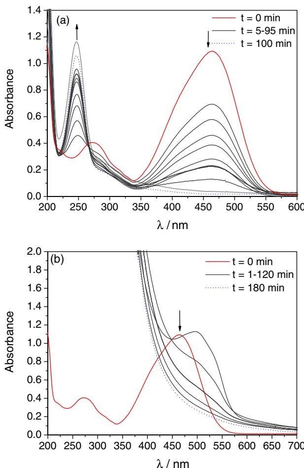
**Figure 6.** Ultraviolet-visible (UV-Vis) spectra of methyl orange ( $5.0 \times 10^{-5}$  mol L<sup>-1</sup>) degradation at 25 °C, pH 5.0, with (a) <sup>50%</sup>Fe/SiO<sub>2</sub> (132.0 mg); and (b) <sup>YM2</sup>Fe/SiO<sub>2</sub> (40.0 mg), H<sub>2</sub>O<sub>2</sub> (0.56 mol L<sup>-1</sup>). The arrows indicate the direction of the band variation.
