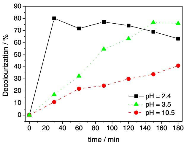
**Figure 11.** Decolorization of methyl orange ( $5.0 \times 10^{-5} \text{ mol L}^{-1}$ ) at different initial pH values using 60 mg of  ${}^{\text{YM}2}\text{Fe}/\text{SiO}_2$  and  $\text{H}_2\text{O}_2$  (0.56 mol L<sup>-1</sup>) at 25 °C.
