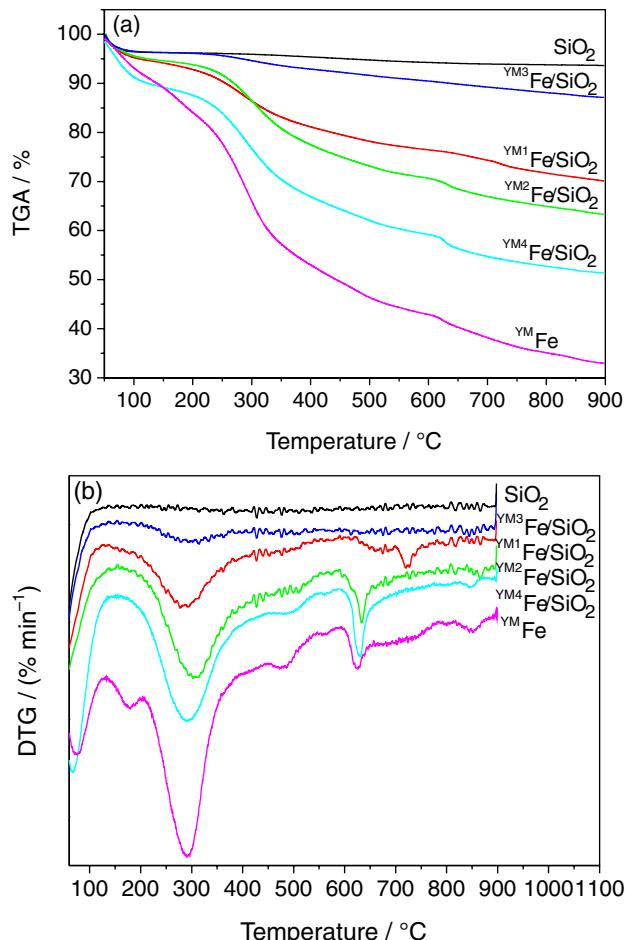
**Figure 5.** (a) Thermogravimetric (TGA) and (b) derivative thermogravimetric analysis (DTG) curves of the Fe/SiO<sub>2</sub> catalysts prepared with yerba mate tea extract.
