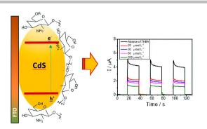
Graphical Abstract Photoelectrochemical (PEC) determination of 3,4,5-trihydroxybenzoic (THBA) with the p-DG-CdS/fluorine-doped tin oxide (FTO) sensor.
