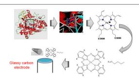
**Graphical Abstract** Modification of glassy carbon electrode with MWCNT-COOH and copper phthalocyanine complex, which is responsible for imitating the active site of the P450 enzyme, iron protoporphyrin IX
